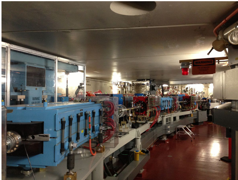
Figure 1.3. The electron storage ring of the Advanced Light Source, Lawrence Berkeley National Laboratory. Dipole magnets (painted blue) steer the beam around the ring, while quadrupole magnets (red) provide focusing to control the beam size. Image courtesy of the Advanced Light Source, by SPat, CC BY-SA 3.0, https://commons.wikimedia.org/w/index.php?curid=25940137 .
