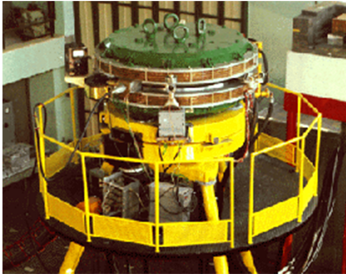
Figure 1.1. AdA (Anello di Accumulazione), the first electron–positron collider. AdA had a diameter of about 1.3 m, and stored beams with energy 250 MeV. It was constructed in Frascati, Italy, in 1961.
