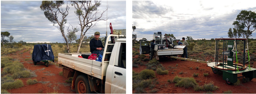
Figure A10. The first EM ELF gradiometer field trial with Regis Resources Pty Ltd commenced in July 2009 in a regional outback Australia in relatively difficult terrain. The monitoring system (CPU, oscilloscope, power amplifier, adjustable power supply, laptop) powered by a small generator was temporarily set up in the back of a Landcruiser trayback. This was connected to the transmitter-receiver unit, which was towed 5 metres behind the vehicle, mounted on the woodentrolley. The results of the field tests have been positive. The system was able to identify known EM conducting targets in the trial area and a number of anomalies were detected in the data collected in an area where geochemical signatures had indicated the likely potential of a massive nickel sulphide deposit. Participants: Jens Balkau (Regis Resources), Tara French (Regis Resources), Nathan Litchfield (Regis Resources) and Alexey Veryaskin (Trinity Research Labs/UWA).
