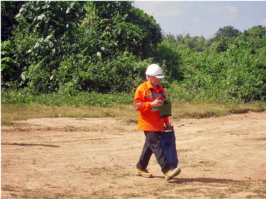
Figure A11. The author testing a handheld EM ELFIS™ gradiometer in Sepon (Laos) that was developed for UXO detection in 2012.
