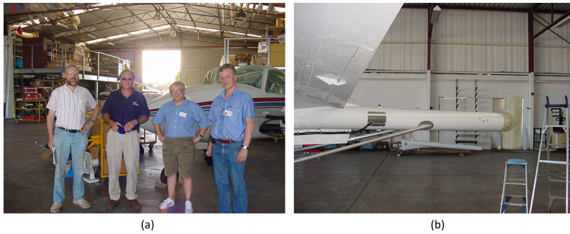
Figure A4. Gravitec's direct string magnetic gradiometer being prepared for flight tests at FUGRO's hangar at Perth's Jandakot airport left to right: Michael Asten (BHP), Howard Golden (WMC), Alexey Veryaskin (Gravitec) and Peter Wolfgram (FUGRO Airborne Services 2003). (b) The magnetic gradiometer assembly is installed in the vertical 'stinger' section attached to the tale of a Cessna plane.
