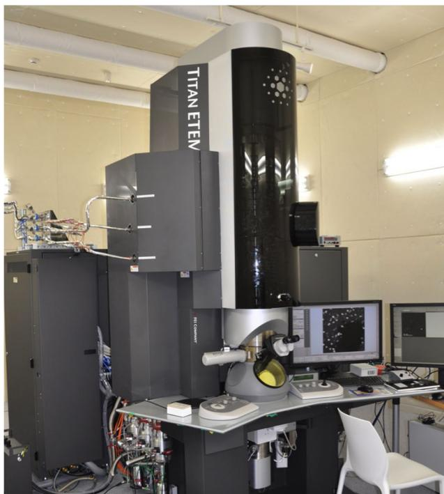
**Figure 1.9.** TEM used for the characterization of NPs presented in this book. (Credit: OIST-Graduate University).
