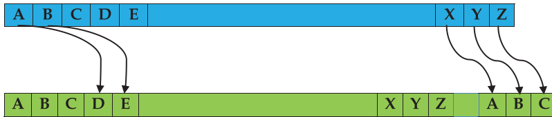
Figure 1.1. Example of character substitution based on Caesar’s algorithm.
