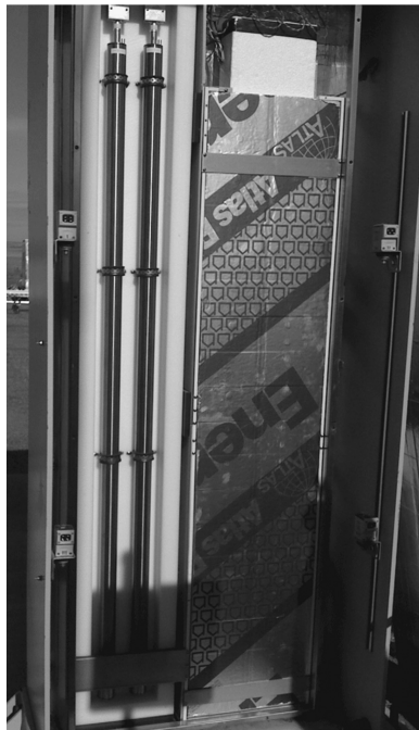
Figure 9.17. Two ^3\text{He} tubes mounted within neutron-moderating material as a radiation portal monitor (RPM). (Reprinted from [34] with the permission of Elsevier.)
