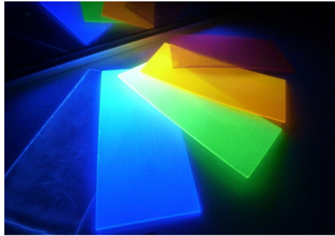
Figure 9.10. Plastic scintillators with different wavelength emission when illuminated with ultraviolet light. (Reprinted from [14] with the permission of Elsevier under Creative Commons License.)
