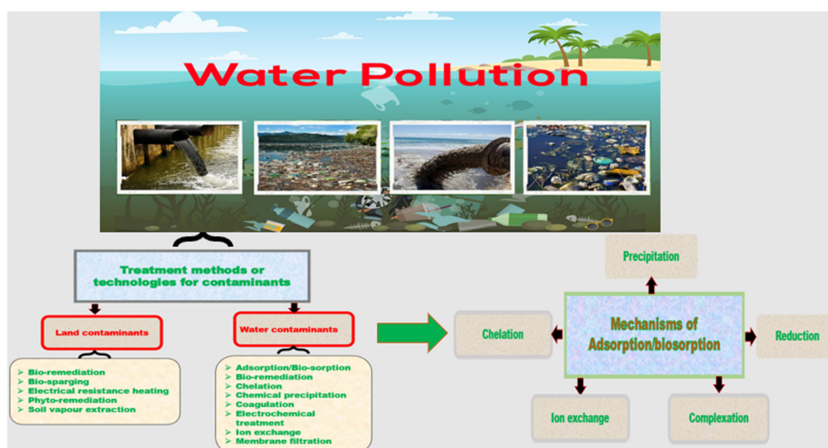
Figure 1.2. A schematic illustration of a variety of pollutant mitigation methods and their relationships to water purification AST (or biosorption) mechanisms. Reprinted by permission from Springer Nature [31], Copyright (2023).
