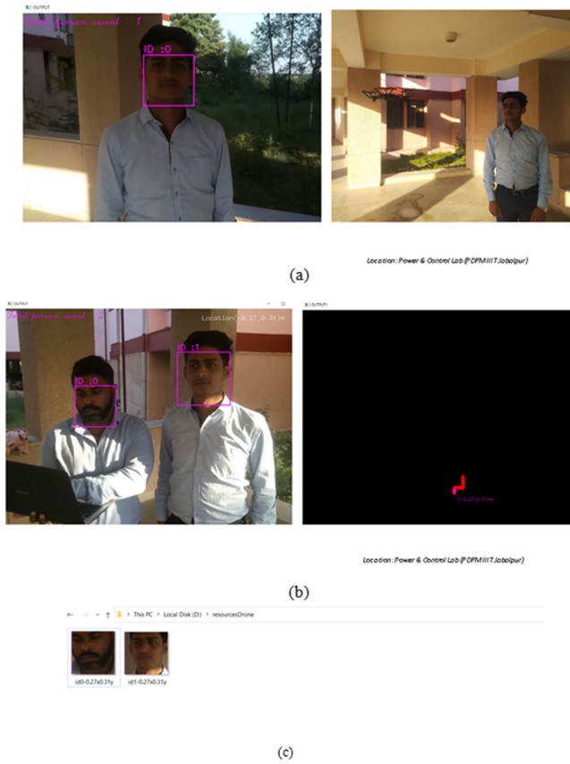
Figure 1.20. Results of the proposed system. (a) Localization and counting of people performed by the proposed system. (b) Tracing the path of the drone. (c) Saving images of people to the database.
