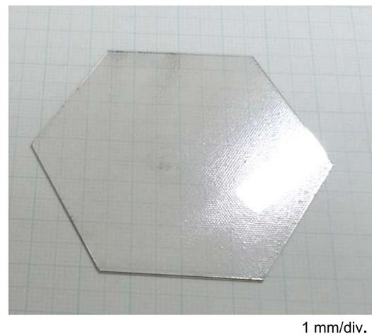
**Fig. 22.** (Color online) Free-standing GaN wafer with a high transparency and 2 in diameter obtained following backgrounding of the first- and second-growth sectors and the application of a chemical mechanical polishing process.
