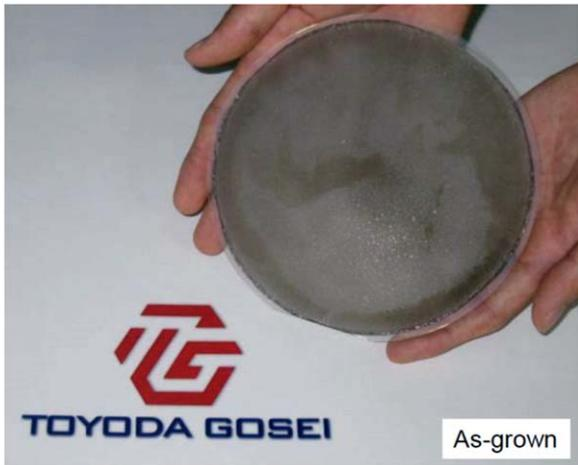
**Fig. 7.** (Color online) Six-inch GaN crystal grown on MOCVD-GaN substrate using Na-flux method. Reprinted from Ref. 8 with permission from Elsevier.
