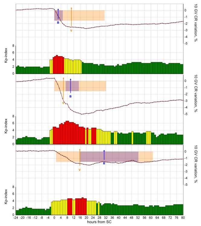
Figure 7. Behavior of averaged CR variations with a rigidity of 10 GV and the Kp index of the geomagnetic activity for different subgroups (Early, Medium, Late—top, middle, and bottom panels, respectively) obtained by the epoch method (zero hour is the hour with SSC). The arrows indicate the average value for each group, and their position on the plot refers to the time of maximum for the IMF intensity and the SW speed, respectively.
