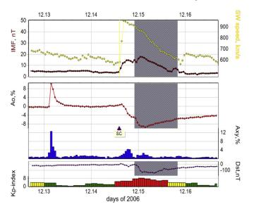
**Figure 5.** Event on 2006 December 13–16. From top to bottom: the SW speed  $[\text{km s}^{-1}]$  and the magnitude of the IMF intensity [nT], the variation in the CR density [A0, %] and the equatorial component of the CR vector anisotropy  $[A_{xy}, \%]$ , and the evolution of the geomagnetic indices (Dst and Kp). The gray shaded area marks the duration of the MC; the vertical green line indicates the timing of the SSC.
