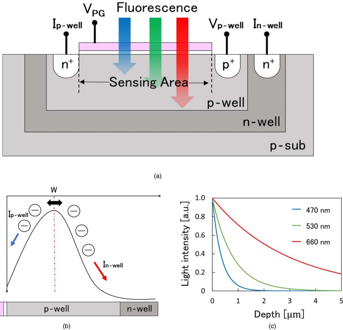
**Fig. 1.** (Color online) Photogate-type optical sensor: (a) cross-sectional diagram, (b) schematic diagram of potential, (c) light intensity attenuation characteristic versus light penetration depth.
