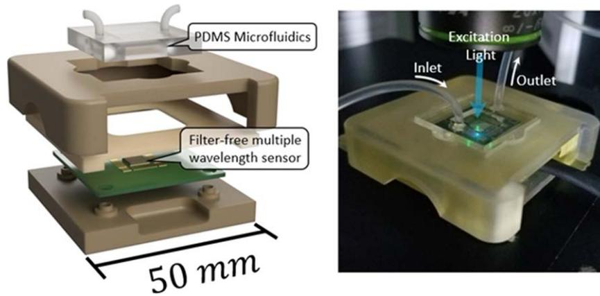
Fig. 7. (Color online) Photos of the 3D design (left) and the fabricated bacteria detection system (right).
