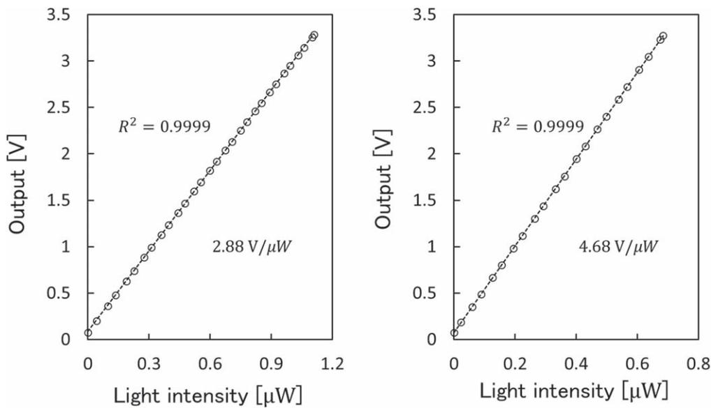
Fig. 4. Output voltage versus input power for blue (left) and red (right) light. The applied photogate voltage was 3 V. An LED light source with wavelengths of 470 nm and 660 nm was irradiated through a 400  $\mu\text{m}$  diameter optical fiber and a 20 $\times$  objective lens.
