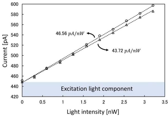
**Fig. 5.** (Color online) Incident light intensity versus output characteristics when simulating fluorescence with an LED light source ( $\lambda_{365\text{ nm}}$ , 1 nW +  $\lambda_{660\text{ nm}}$ , 0–3 nW). The open circles and open triangles stand for the cases with photogate voltages of 3 V and 1 V, respectively.
