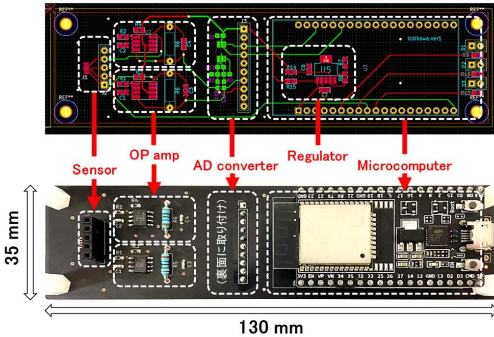
Fig. 3. (Color online) Photo of fabricated circuits.
