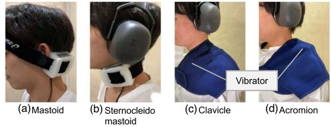
**Fig. 5.** (Color online) Fixed locations of the vibrator in the experiments. An elastic band with foam was used to fix the vibrator to the (a) mastoid process and (b) sternocleidomastoid muscle, and an icing supporter was using to fix the vibrator to the (c) clavicle and (d) acromion.<sup>25)</sup>
