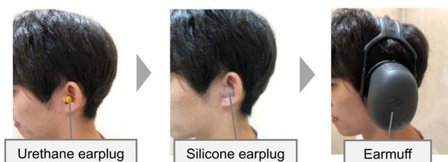
**Fig. 1.** (Color online) Method of insulation of the air-conducted sounds used in the experiments.
