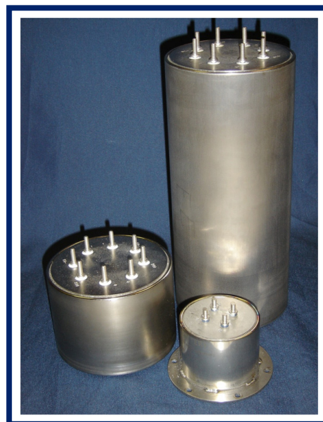
Fig. 2. Various thermal batteries used for powering the entry and descent and landing sequences on the Mars Exploration Rover and Mars Science Laboratory rover missions. These batteries incorporate pyrotechnic devices to activate the cells and generate the molten electrolyte.
