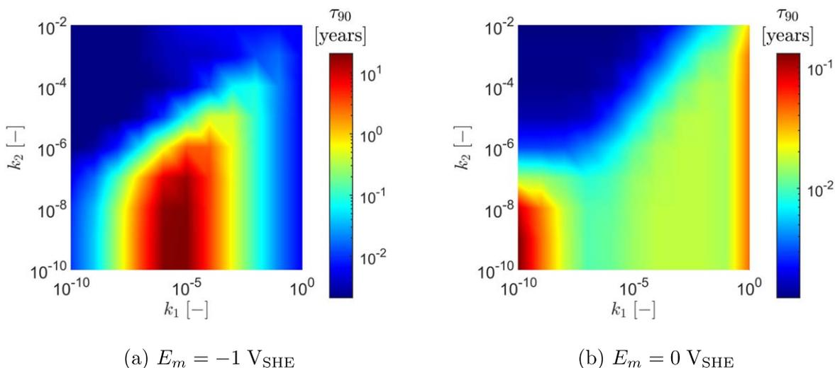
**Figure 8.** Influence of the Volmer and Heyrovsky reaction rate constants on the time required to reach 90% of the final (steady state) average lattice hydrogen concentration. As elaborated in the text, the reaction rate constant  $k_1$  is defined to consistently vary the Volmer reaction rates, while the reaction rate constant  $k_2$  refers to the Heyrovsky reaction rates.
