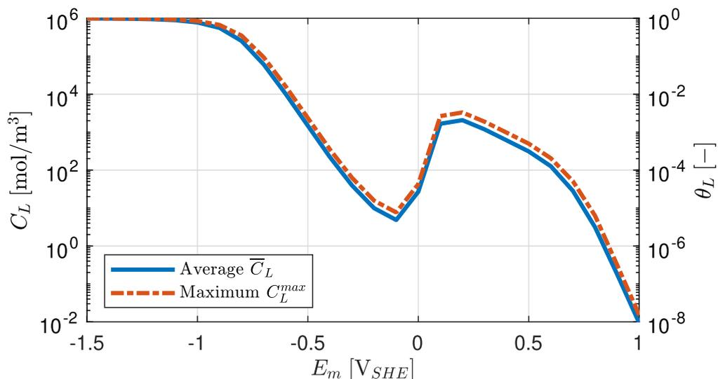
**Figure 10.** Influence of the applied potential  $E_m$  on hydrogen uptake; steady state predictions of lattice hydrogen concentration (left) and occupancy (right). Results are shown for the maximum ( $C_L^{\max}$ , orange dashed line) and average ( $\bar{C}_L$ , blue solid line) hydrogen concentrations at equilibrium.
