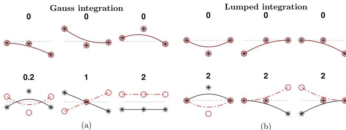
**Figure 2.** Eigenvalues and modes obtained for the matrices from Eq. 52 using: (a) a Gauss integration scheme, and (b) the lumped integration scheme. Red dashed lines are used for the changes in lattice hydrogen concentration, while black lines are used for the changes in surface occupancy relative to the zero concentration and occupancy (gray dotted lines). Red circles and black stars indicate the values within the nodes.
