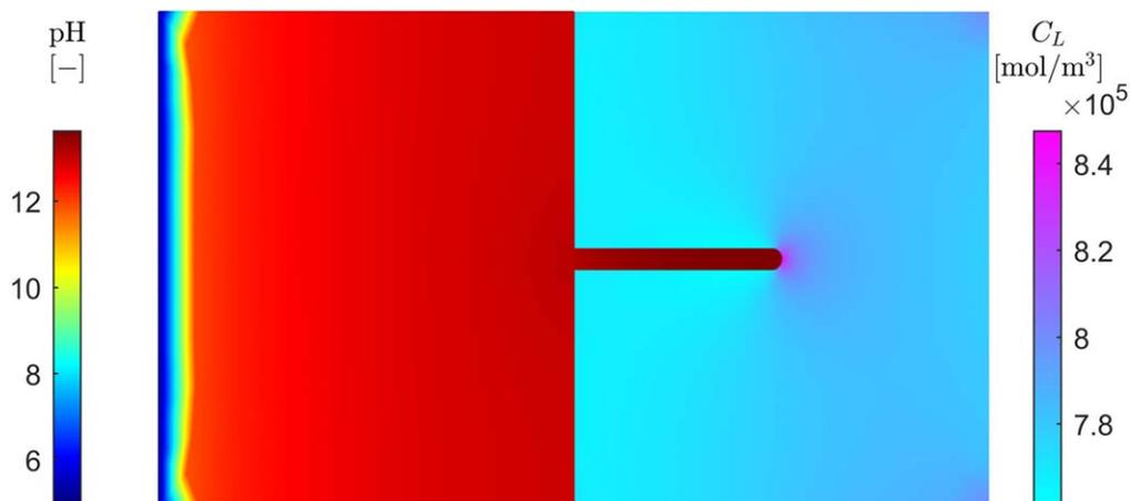
**Figure 5.** Contours of the electrolyte pH (left) and the lattice hydrogen concentration  $C_L$  in the metal (right). The results are predicted for an applied potential of  $E_m = -1 \text{ V}_{\text{SHE}}$  and at steady state ( $t = 50$  years).
