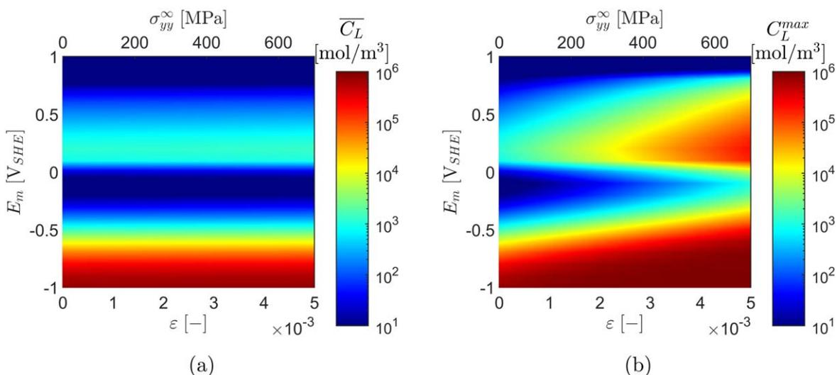
**Figure 13.** Hydrogen uptake sensitivity to mechanical straining. Steady state results for the blunted crack case showing: (a) the average lattice hydrogen concentration  $\bar{C}_L$ , and (b) the maximum hydrogen concentration  $C_L^{\max}$  as a function of the remote strain/stress and the applied potential  $E_m$ .
