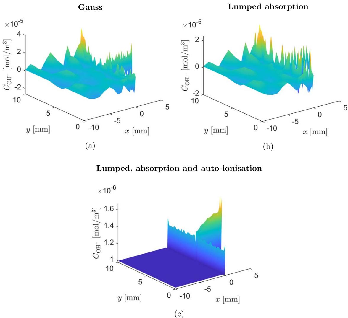
**Figure 4.** Comparison of lumped and Gaussian integration by assessing their effect on the  $\text{OH}^-$  concentration after a single iteration using  $\Delta t = 1$  s, and  $k_4 = 10^3 \text{ m s}^{-1}$ ; (a) Gauss integration, (b) lumped integration for the absorption reaction, and (c) lumped integration for the absorption and auto-ionisation reactions.
