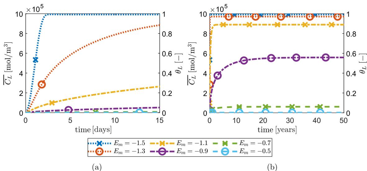
**Figure 9.** Influence of the applied potential  $E_m$  (in  $\text{V}_{\text{SHE}}$ ) on hydrogen uptake; evolution of the average lattice hydrogen concentration  $\bar{C}_L$  (a) over the first 15 d, and (b) over 50 years.
