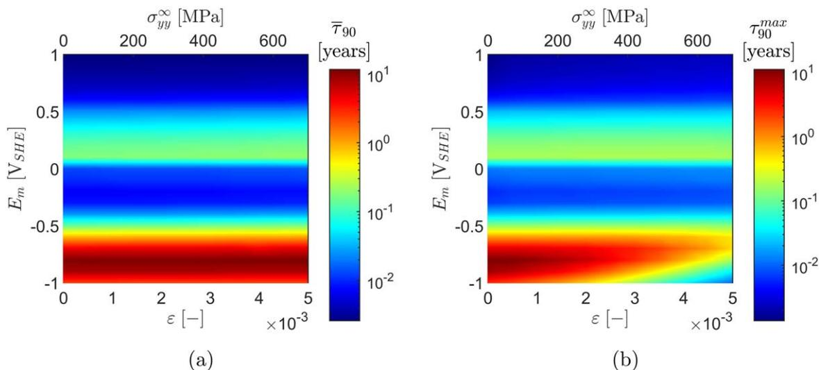
**Figure 14.** Hydrogen uptake sensitivity to mechanical straining. Time required to attain 90% of the steady state values of (a) the average lattice hydrogen concentration  $\bar{C}_L$ , and (b) the maximum hydrogen concentration  $C_L^{max}$ . The results have been obtained for the blunted crack case, as a function of the remote strain/stress and the applied potential  $E_m$ .
