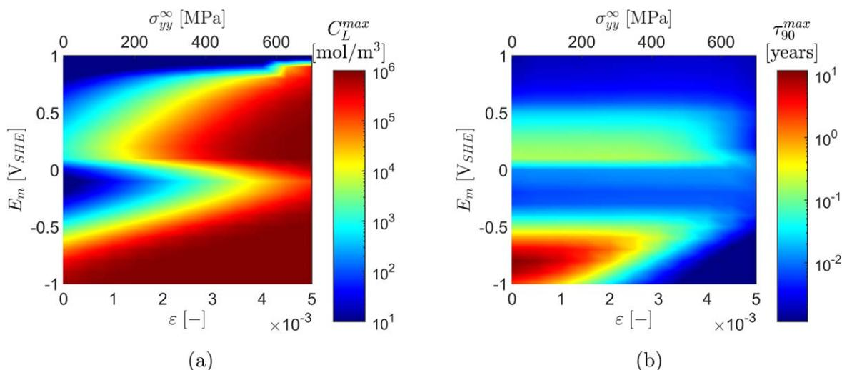
**Figure 15.** Hydrogen uptake sensitivity to mechanical straining. Results obtained for the sharp crack case as a function of the applied load and potential, showing: (a) the maximum lattice hydrogen concentration  $C_L^{max}$  at steady state, and (b) the time required to attain 90% of this steady state  $C_L^{max}$ .
