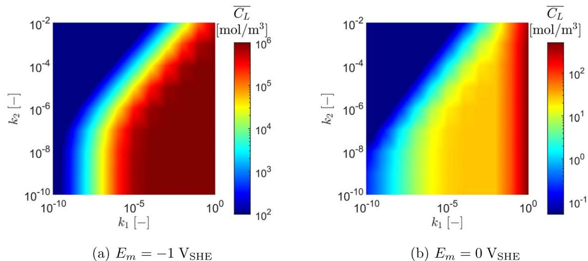
**Figure 7.** Influence of the Volmer and Heyrovsky reaction rate constants on the average lattice hydrogen concentration  $\bar{C}_L$  at  $t = 50$  years. As elaborated in the text, the reaction rate constant  $k_1$  is defined to consistently vary the Volmer reaction rates, while the reaction rate constant  $k_2$  refers to the Heyrovsky reaction rates.
