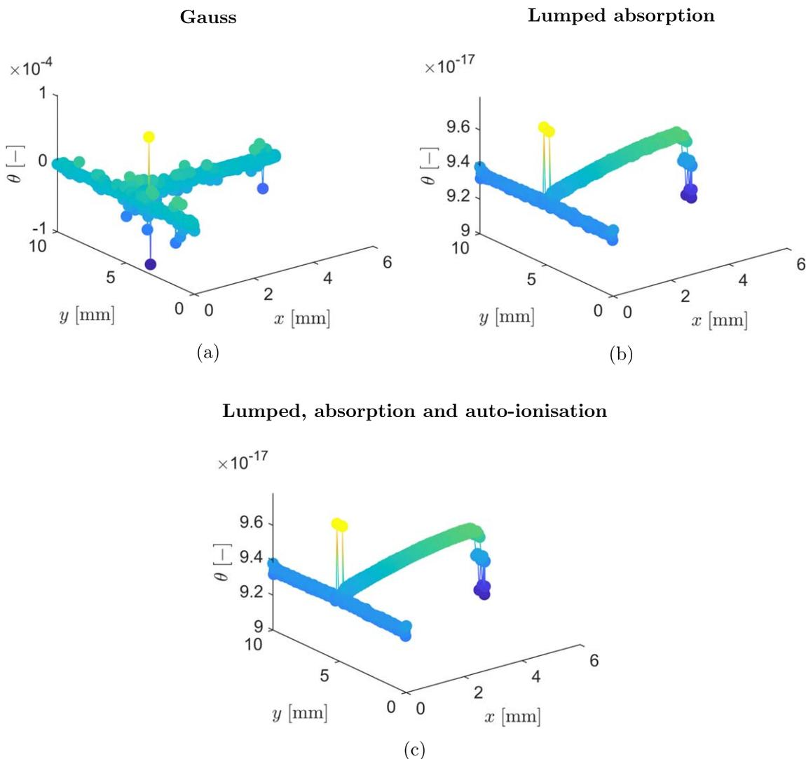
**Figure 3.** Comparison of lumped and Gaussian integration by assessing their effect on the hydrogen surface coverage  $\theta$  after a single iteration using  $\Delta t = 1$  s, and  $k_A = 10^3$  m s<sup>-1</sup>; (a) Gauss integration, (b) lumped integration for the absorption reaction, and (c) lumped integration for the absorption and auto-ionisation reactions.
