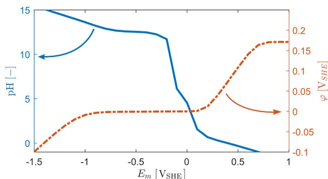
**Figure 11.** Sensitivity of the environmental conditions at the crack tip to the applied potential  $E_m$ . The left axis shows the change in electrolyte pH (blue solid curve), while the right axis denotes the variation in electrolyte potential  $\phi$  (red dashed curve).
