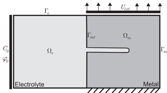
**Figure 1.** Overview of domain considered, composed of the electrolyte sub-domain  $\Omega_e$  with external boundary  $\Gamma_e$ , metal sub-domain  $\Omega_m$  with external boundary  $\Gamma_m$ , and the electrolyte-metal interface  $\Gamma_{int}$ .
