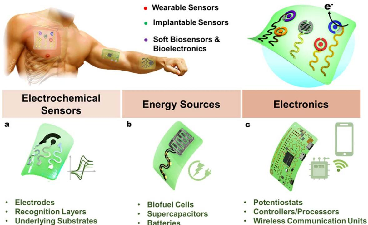
**Figure 1.** Conceptual illustration of flexible and stretchable electrochemical sensing systems that allow key capabilities for biological material–sensor interface in biomedical applications, such as wearable and implantable platforms. The flexible and stretchable electrochemical sensing systems consist of (a) sensors; (b) energy sources; and (c) electronics.
