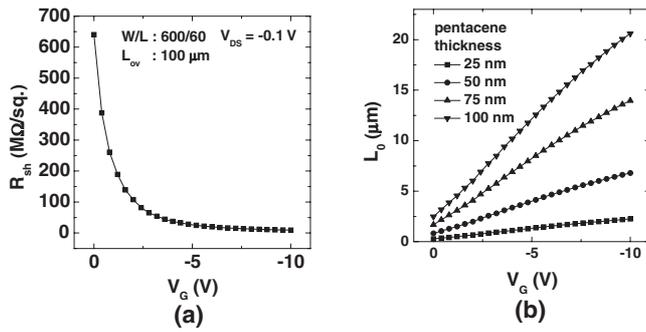
Fig. 7. (a)  $R_{sh}$  of the fabricated OTFTs obtained from  $I$ - $V$  characteristics of 25 nm device. (b)  $L_0$  of the fabricated devices which are calculated with eq. (8).  $L_0$  is always smaller than the overlap length  $L_{ov} = 100 \mu\text{m}$ .
