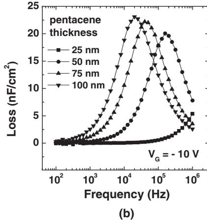
Fig. 6. (a) The model used for the admittance modeling is composed of the insulator capacitance  $C_i$ , the semiconductor capacitance  $C_s$ , the bulk capacitance  $C_B$ , the bulk resistance  $R_B$ , and the external series resistance  $R_{ext}$ . (b) The peaks of the loss curves shift to the low frequency due to the large bulk resistance of the thick pentacene film.
