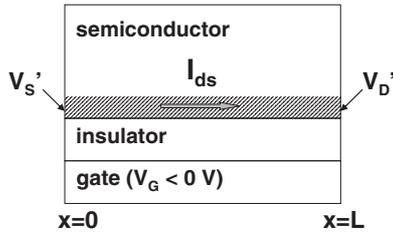
Fig. 2. For the channel, the current is determined by  $R_{sh}$  and the intrinsic source and drain voltage, i.e.,  $V_S'$  and  $V_D'$ .
