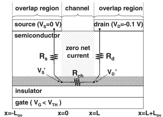
Fig. 1. Cross-section of a top-contact OTFT in the linear region. Accumulation layer is induced uniformly at the bottom of semiconductor due to the negative  $V_G$ .  $V_S'$  and  $V_D'$  represent intrinsic source and drain voltage, respectively.  $R_s$ ,  $R_d$ , and  $R_{ch}$  denote source, drain, and channel resistance, respectively.
