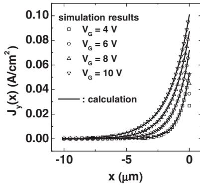
Fig. 4. To verify eq. (5),  $J_y(x)$  is obtained from the simulation on an amorphous Si (a-Si) TFT. Good agreement between simulation and calculation confirms that the equation for  $J_y(x)$  is properly derived. For the simulation, oxide of 45 nm and a-Si of 250 nm is used for the a-Si TFT. The channel length of the device is 10  $\mu\text{m}$ .
