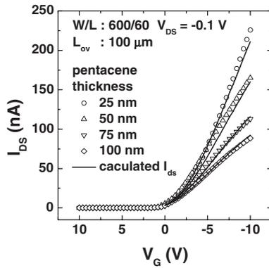
Fig. 8. Measured  $I$ - $V$  curve (dotted line) and the calculated  $I$ - $V$  curve (solid line) using eq. (12) show good agreement.
