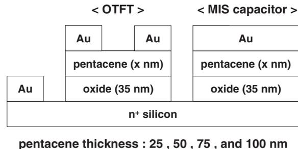
Fig. 5. Structure of the fabricated OTFTs and MIS capacitors. Pentacene thicknesses are varied to obtain different  $R_y$ . Gate-source overlap length  $L_{ov}$  is fixed to 100  $\mu\text{m}$ .
