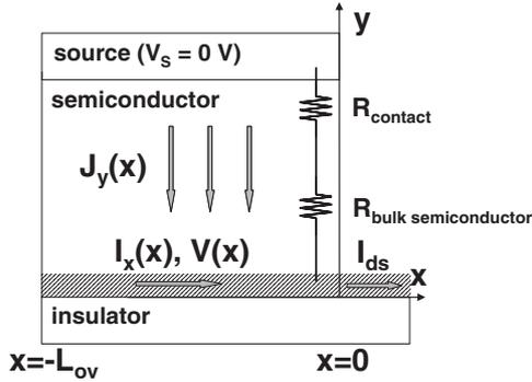
Fig. 3. For the overlap region,  $I_x(x)$ ,  $V(x)$ , and  $J_y(x)$  are determined by  $R_{sh}$ ,  $R_y$  and Kirchhoff's law. For the current continuity,  $I_x(x)$  becomes  $I_{ds}$  at  $x = 0$ .
