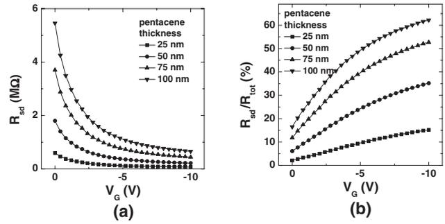
Fig. 9. (a) Obtained  $R_{sd}$  using eq. (9) for the fabricated OTFTs. (b) The ratio of  $R_{sd}$  to the total resistance is as large as 60% when the pentacene thickness is 100 nm.
