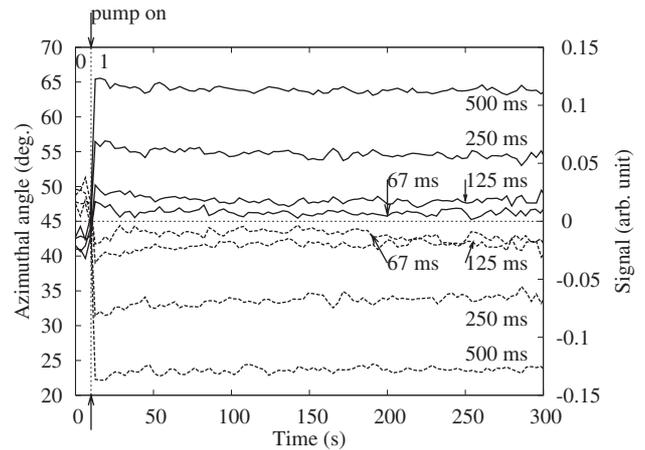
Fig. 6. Recording duration dependence. The recording was started at 10 s. Solid and dashed lines show time evolutions of the azimuthal angle and the signal, respectively.
