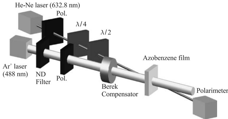
Fig. 4. Experimental setup of polarization recording.
