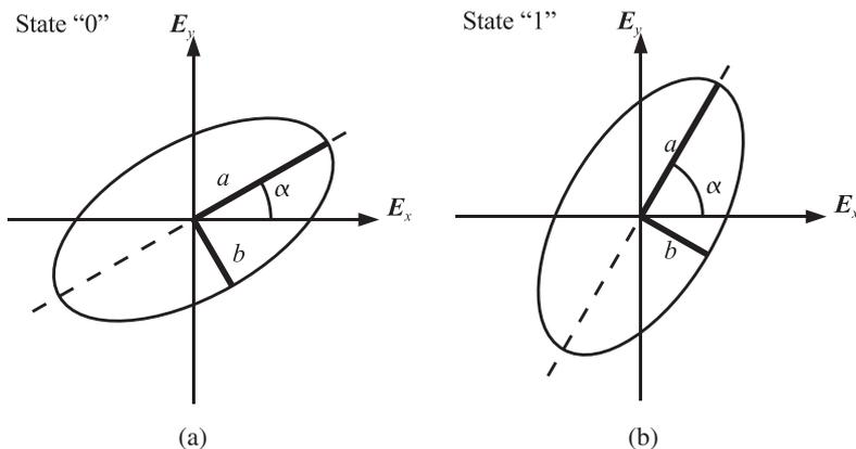
Fig. 2. States of elliptical polarization. (a) and (b) show the polarization ellipses of states “0” and “1”, respectively. Here,  $E_x$ ,  $E_y$ ,  $a$ ,  $b$ , and  $\alpha$  are the  $x$ - and  $y$ -components of the electric field, and the long and short radii, and azimuthal angle of the polarization ellipse, respectively.
