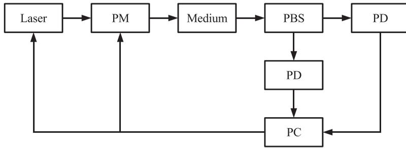
Fig. 3. Feedback system of polarization recording. PM, PBS, and PD are the polarization modulator, polarization beam splitter, and photodetector, respectively.
