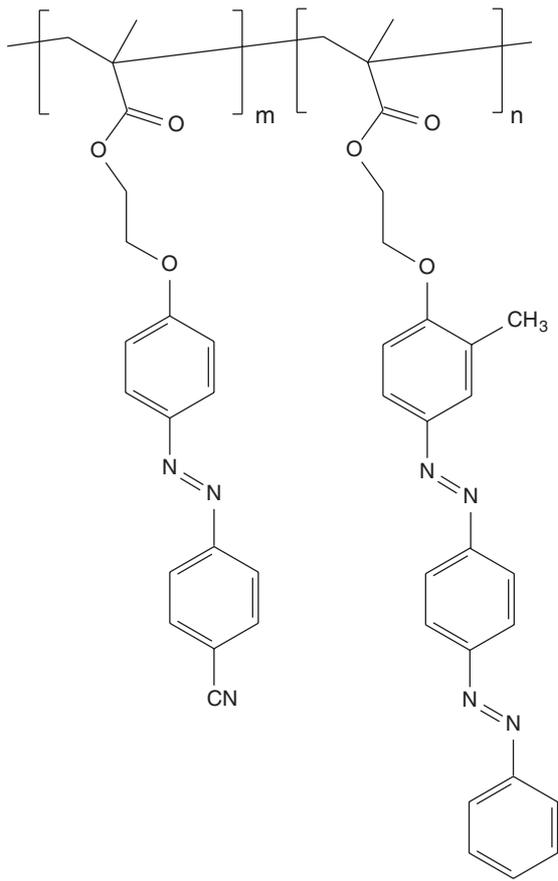
Fig. 1. Chemical structure of PCDY copolymer. The ratio of  $m : n$  is 1 : 1 in PCDY50.
