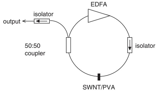
Fig. 4. Laser configuration constituting a ring cavity made of single-mode fibers and optical components.
