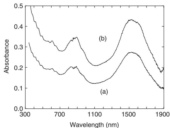
Fig. 1. Optical absorption spectra of the SWNT/PVA films: (a) 30- $\mu\text{m}$ -thick film used in the mode-locking laser experiment, (b) 100- $\mu\text{m}$ -thick film used in the ASE suppression experiment.
