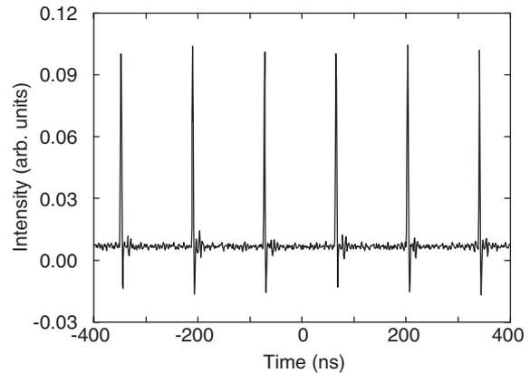
Fig. 5. Repetition of the single-pulse mode-locked lasing. Repetition rate was 7.26 MHz.
