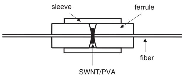
Fig. 3. Mode-locking device structure using a SWNT/PVA film. This diagram is a close-up of the essential part inside a FC adaptor. The ferrules are pushed by springs from both sides.
