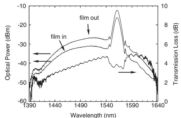
Fig. 10. Transmission loss spectrum of a SWNT/PVA composite film measured with ASE plus femtosecond light source. Light source spectra are also shown.
