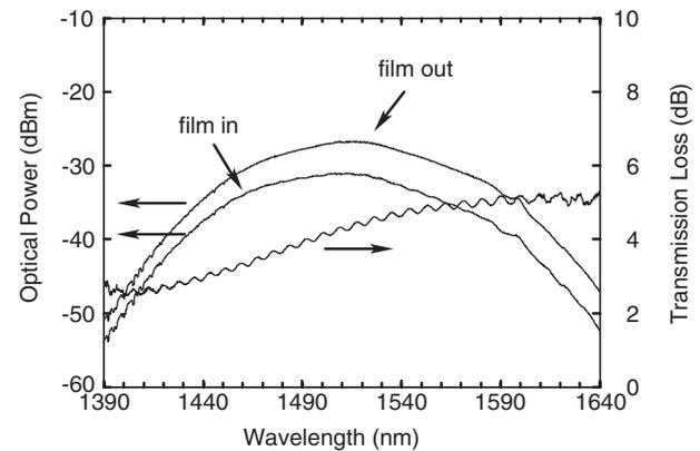
Fig. 9. Transmission loss spectrum of a SWNT/PVA composite film measured with ASE light source. ASE spectra are also shown.
