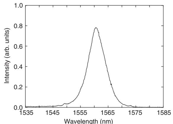
Fig. 6. Output optical spectrum under the mode-locked lasing condition.
