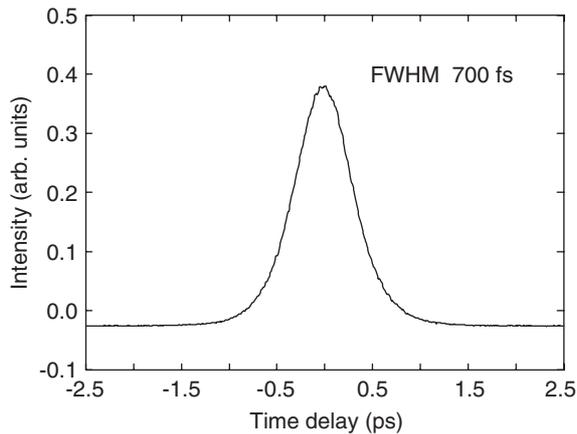
Fig. 7. Autocorrelation trace under the mode-locked lasing condition.
