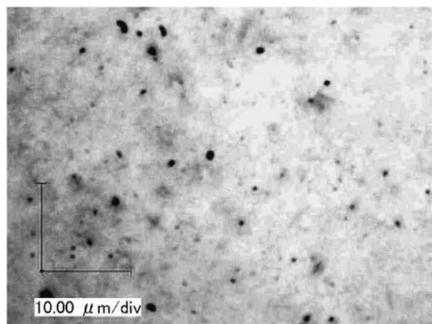
Fig. 2. Optical microscope image of a 30- $\mu\text{m}$ -thick SWNT/PVA film fabricated using NaDDBS surfactant.
