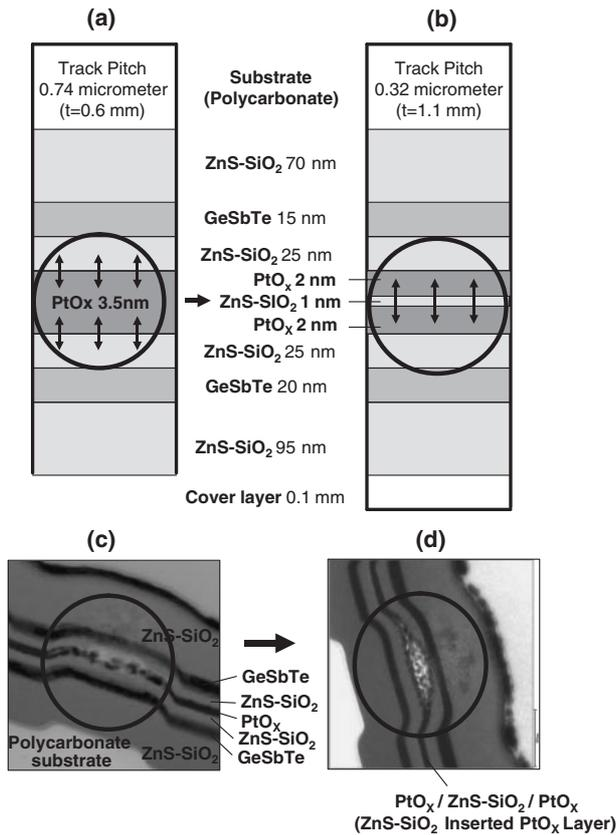
Fig. 1. Sample structure and radial direction TEM images: (a) conventional structure with PtO<sub>x</sub> single layer, (b) new structure with ZnS-SiO<sub>2</sub>-inserted PtO<sub>x</sub> layer, (c) unclear 75 nm mark shape of conventional structure and (d) clear 75 nm mark shape of blue structure.
