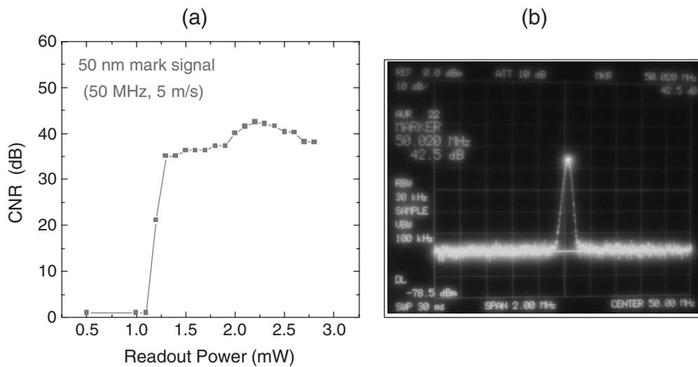
Fig. 4. Threshold characteristics and 50 nm CNR of the sample disk: (a) readout power dependence and (b) CNR spectrum showing 42.5 dB for 50 nm mark signal.
