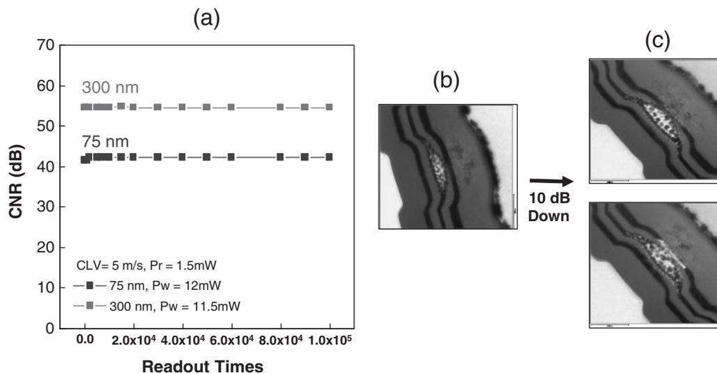
Fig. 5. Stability characteristics and deterioration mechanism: (a) readout stability, (b) initial state of CNR 43 dB and (c) deteriorated states of CNR 33 dB after 100 times of 3.5 mW reading.
