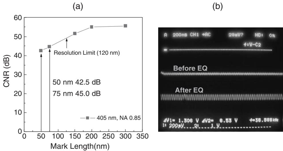
Fig. 3. Signal characteristics of the sample disks: (a) frequency response and (b) RF waveform of 75 nm mark signal.
