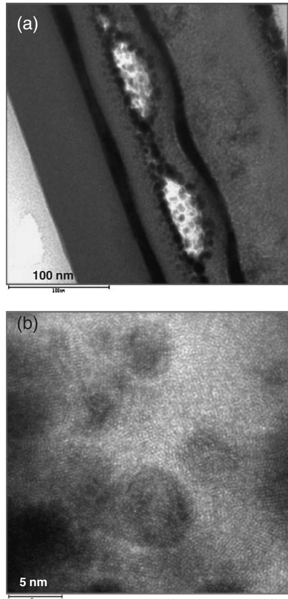
Fig. 2. Cross-sectional TEM images: (a) track direction cross-sectional TEM image showing bubble and (b) atom arrangement inside the bubbles.
