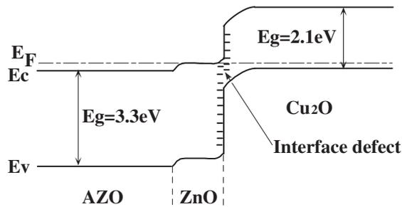
Fig. 3. Energy band diagram of the AZO/ZO/Cu<sub>2</sub>O structure.
