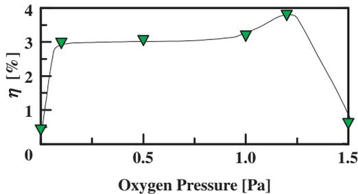
Fig. 4.  $\eta$  as a function of the O<sub>2</sub> gas pressure used for depositing the ZO thin-film layer in AZO/ZO/Cu<sub>2</sub>O solar cells.
