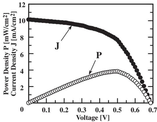
**Fig. 1.**  $J$ - $V$  and  $P$ - $V$  characteristics of an AZO/ZO/Cu<sub>2</sub>O solar cell fabricated with a 50-nm-thick ZO thin-film layer prepared at an O<sub>2</sub> gas pressure of 1.2 Pa.
