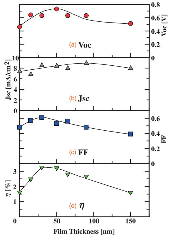
**Fig. 2.**  $V_{OC}$ ,  $J_{SC}$ , FF, and  $\eta$  as functions of the ZO thin-film layer thickness in AZO/ZO/Cu<sub>2</sub>O solar cells.
