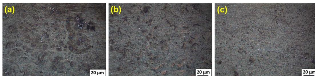
**Figure 14.** Corroded images (a) base alloy, (b) PP-FSP, and (c) IP-FSP samples.
