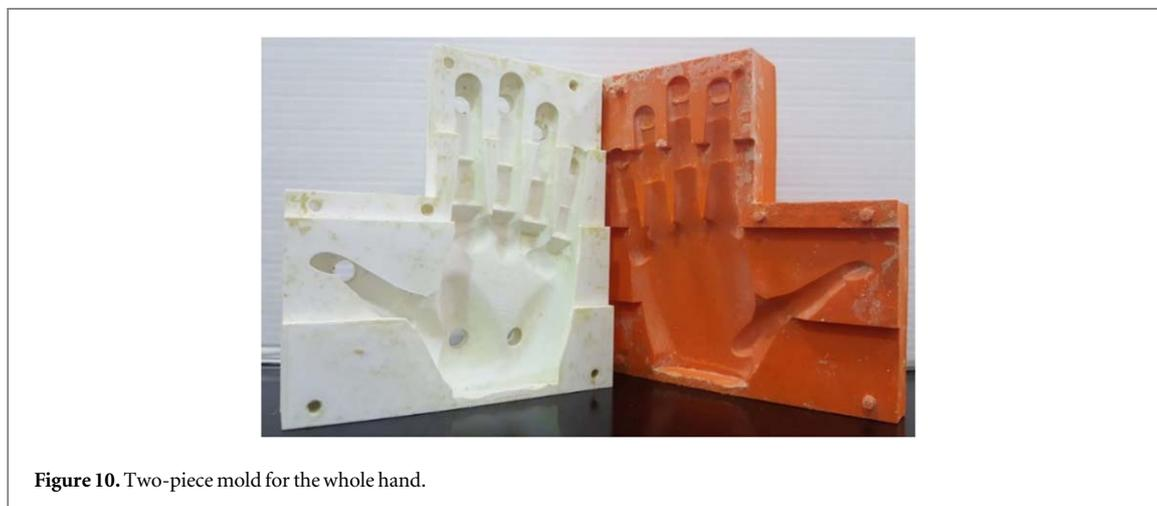
**Figure 10.** Two-piece mold for the whole hand.
