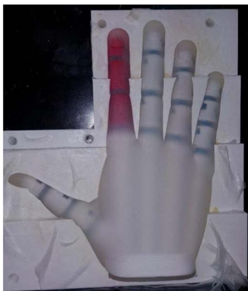
**Figure 12.** Cured hand in the bottom mold.
