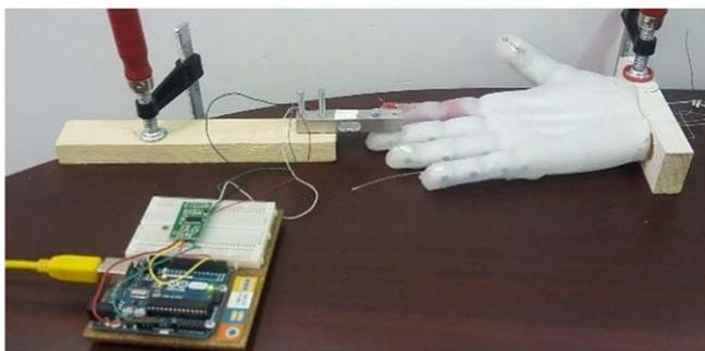
Figure 15. Experimental setup to measure fingertip force.
