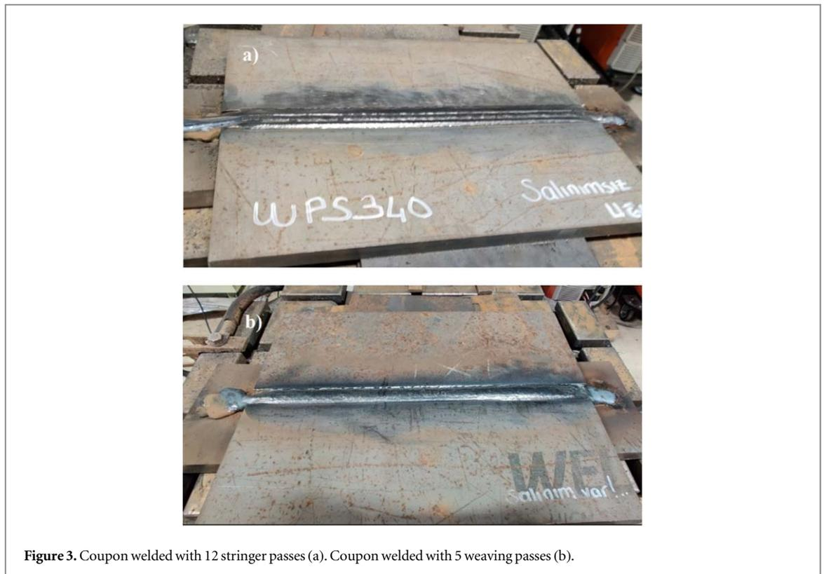
**Figure 3.** Coupon welded with 12 stringer passes (a). Coupon welded with 5 weaving passes (b).
