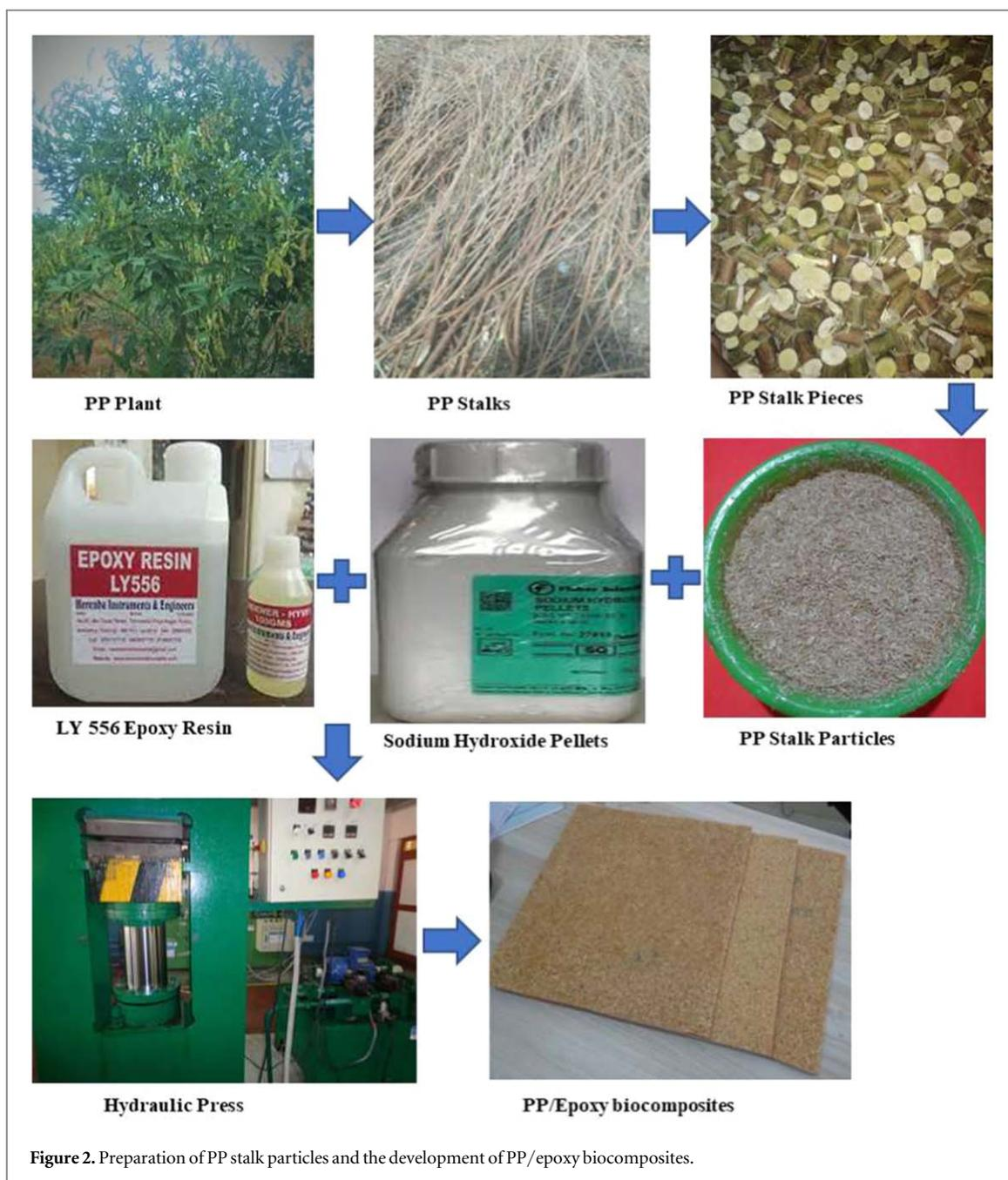
Figure 2. Preparation of PP stalk particles and the development of PP/epoxy biocomposites.
