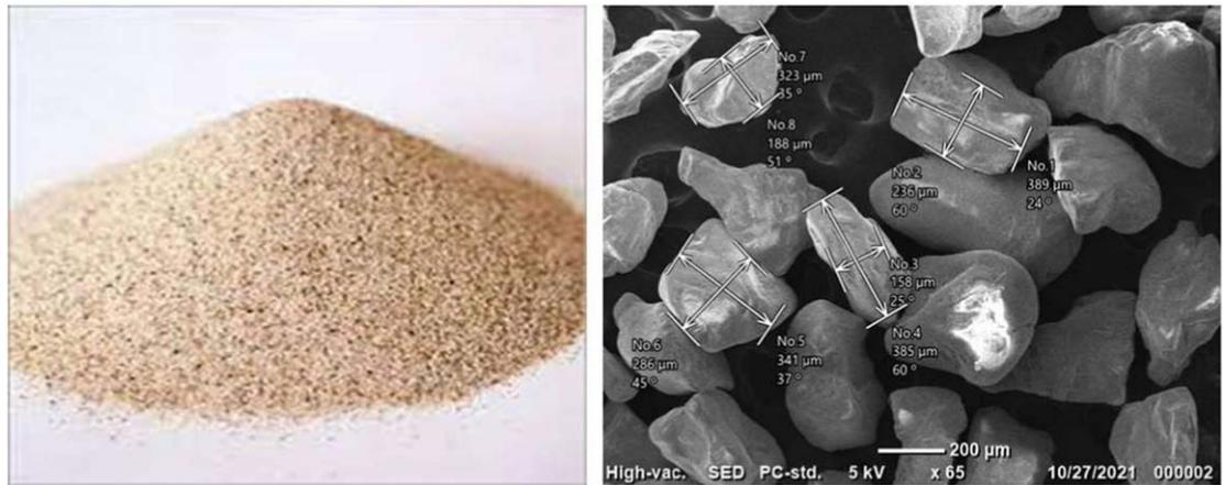
Figure 3. Morphology of silica sand used in three-body abrasive wear testing.
