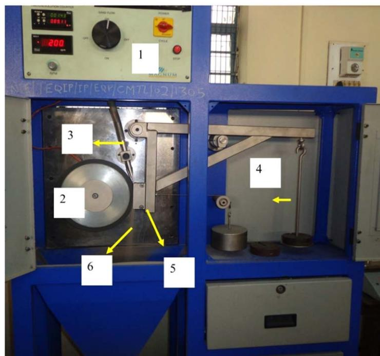
Figure 4. Three-body abrasive wear test rig used in wear testing of PP/epoxy composites.
