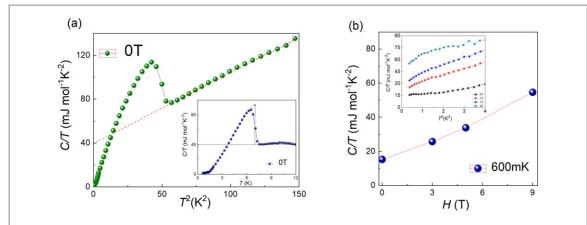
**Figure 5.** (a) Specific heat coefficient C/T of  $Sc_{20}BC_{27}$  as a function of  $T^2$ . The inset shows temperature dependence of the difference electronic specific heat coefficient ( $\Delta C_e/T$ ) between the superconducting and normal states. (b) Magnetic field dependence of the field induced specific heat coefficient C/T of  $Sc_{20}BC_{27}$  at different field in the low temperature.
