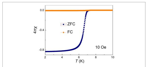
Figure 4. Temperature dependence of the magnetic susceptibility (M/H) measured in the applied field of H=10 Oe. ZFC and FC indicate the zero-field-cooling and field-cooling processes, respectively.
