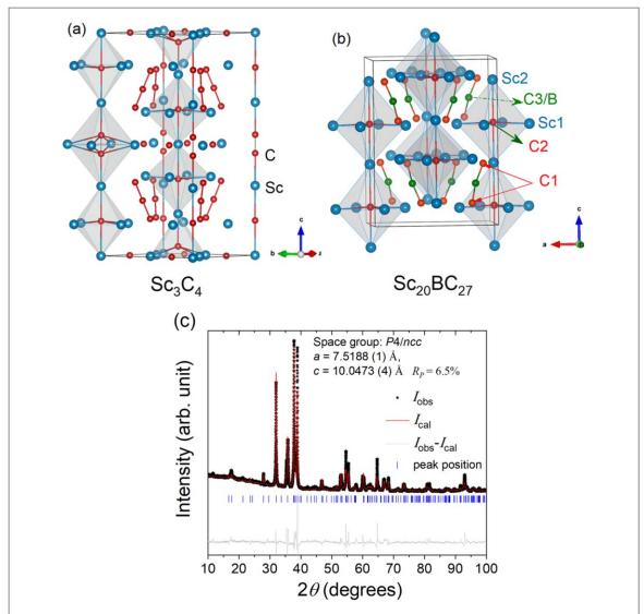
Figure 1. Crystal structures of (a)  $Sc_3C_4$  and (b)  $Sc_{20}BC_{27}$ . (c) Typical Rietveld refinement of  $Sc_{20}BC_{27}$  under ambient conditions. The vertical bars represent the calculated Bragg reflection positions of the diffraction peaks for  $Sc_{20}BC_{27}$ . The difference between the observed (scatters) and the fitted patterns (line) is shown at the bottom of the diffraction peaks.
