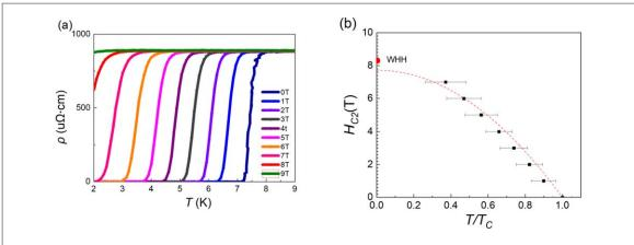
**Figure 3.** (a) Temperature dependence of the resistivity at different fields. (b) Temperature dependence of the upper critical magnetic field. The red solid circle shows the upper critical field obtained from WHH fitting.
