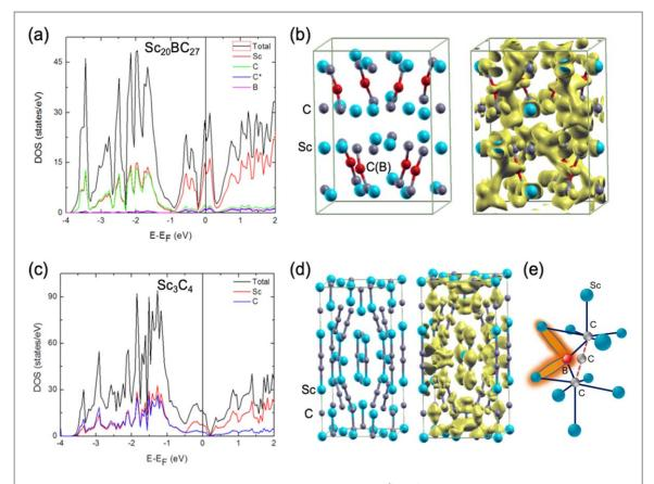
Figure 6. Calculated electronic density of states for (a)  $Sc_{20}BC_{27}$  and (c)  $Sc_3C_4$ . 'C\*' and 'B' denote the middle C and B atoms in the C-C (B)-C fragment of  $Sc_{20}BC_{27}$ . Crystal structure and integrated charge densities in an energy interval [-0.25, 0] eV for (b)  $Sc_{20}BC_{27}$  and (d)  $Sc_3C_4$ . Here the Fermi energy  $E_F$  sets to zero. (e) Schematic coordination of C-C(B)-C fragment.
