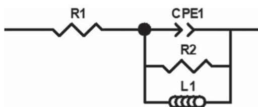
Figure 7. Equivalent circuit to fit electrochemical impedance spectroscopy of as-extruded alloys.
