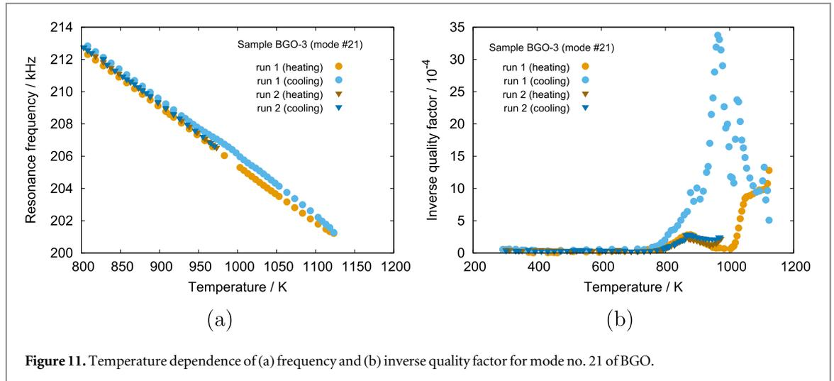
**Figure 11.** Temperature dependence of (a) frequency and (b) inverse quality factor for mode no. 21 of BGO.
