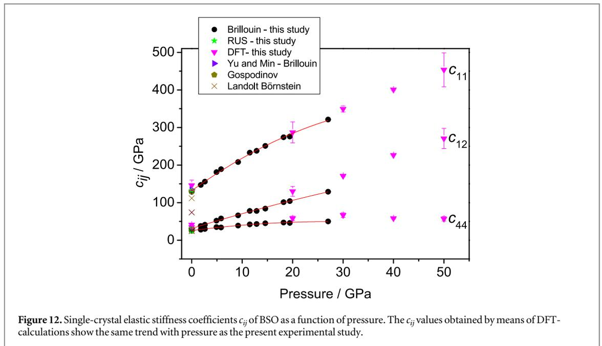
**Figure 12.** Single-crystal elastic stiffness coefficients  $c_{ij}$  of BSO as a function of pressure. The  $c_{ij}$  values obtained by means of DFT-calculations show the same trend with pressure as the present experimental study.
