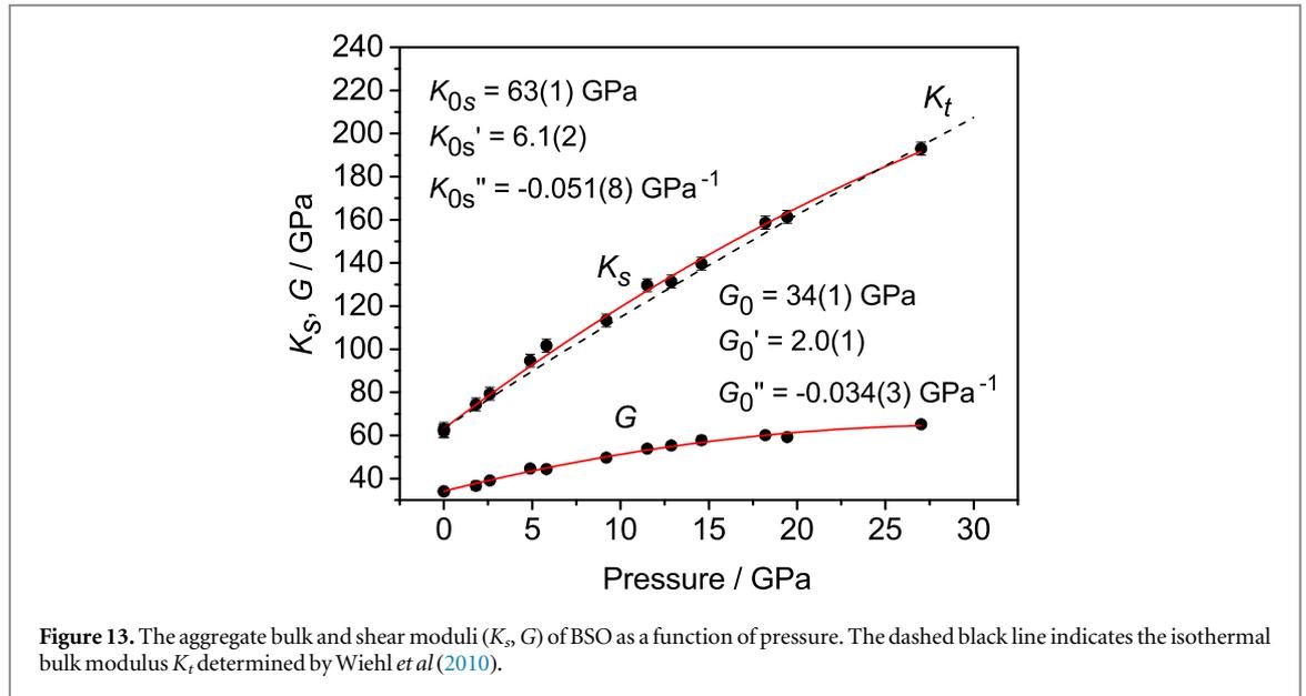
**Figure 13.** The aggregate bulk and shear moduli ( $K_s$ ,  $G$ ) of BSO as a function of pressure. The dashed black line indicates the isothermal bulk modulus  $K_t$  determined by Wiehl *et al* (2010).
