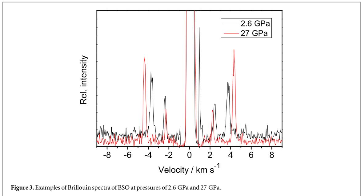
Figure 3. Examples of Brillouin spectra of BSO at pressures of 2.6 GPa and 27 GPa.
