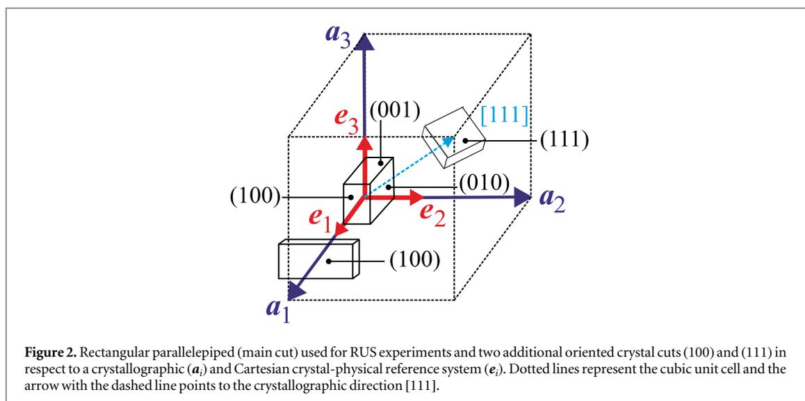
**Figure 2.** Rectangular parallelepiped (main cut) used for RUS experiments and two additional oriented crystal cuts (100) and (111) in respect to a crystallographic ( $a_i$ ) and Cartesian crystal-physical reference system ( $e_i$ ). Dotted lines represent the cubic unit cell and the arrow with the dashed line points to the crystallographic direction [111].
