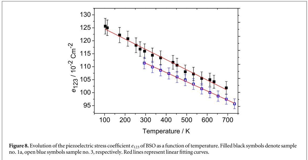
**Figure 8.** Evolution of the piezoelectric stress coefficient  $e_{123}$  of BSO as a function of temperature. Filled black symbols denote sample no. 1a, open blue symbols sample no. 3, respectively. Red lines represent linear fitting curves.
