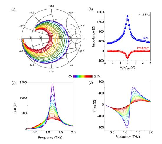
**Figure 4.** Tunable impedance surface. (a) Smith chart representation of the complex THz reflectivity which allows us to extract surface impedance of the device. (b) The variation of both the real (*x*-axis on the chart) and imaginary parts of the impedance at resonance extracted from Smith chart as a function of positive and negative gate voltages. The real (c) and imaginary (d) parts of the complex impedance plotted with respect to frequency.
