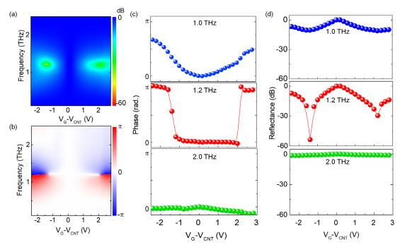
**Figure 3.** Voltage controlled phase. 2D maps showing the variation of the reflection amplitude (a) and the reflection phase (b) as a function of the frequency and the gate voltage. The color bar indicates the values of reflection (dB) and phase (radian). (c) and (d) show the variation of phase and amplitude with the gate voltage for 1.0, 1.2, and 2.0 THz frequencies.
