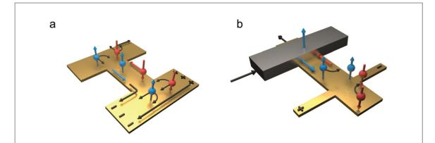
Figure 5. (a) Hall bar device. A charge current in the top arm generates a spin current via the SHE that flows to the bottom bar, which results in a measurable voltage via the inverse SHE. (b) Nonlocal device where the spin current is achieved via spin injection from a ferromagnet (dark electrode). Adapted from [32].
