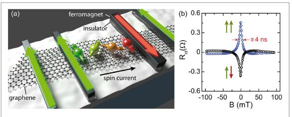
**Figure 1.** (a) Schematics of the typical four-terminal spin valve geometry for measuring spin lifetime in graphene samples. (b) Hanle experimental curve from which spin lifetimes are extracted using a semiclassical spin diffusion equation. Reprinted with permission from [14]. Copyright 2014 American Chemical Society.
