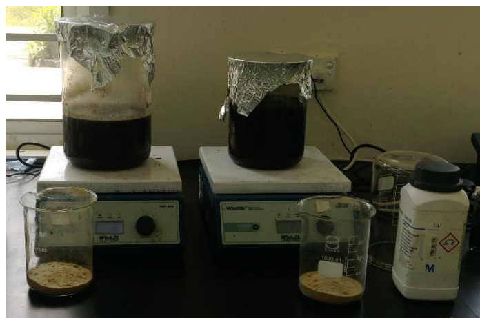
Figure 1. Oily-biological sludge thermo-chemical pre-treatment through magnetic stirrer.
