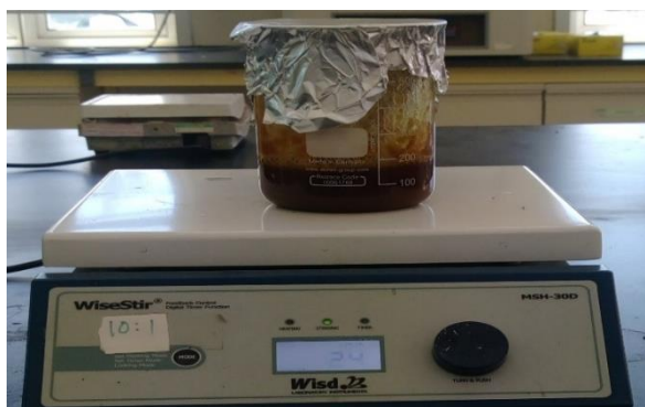
Figure 3. Thermo-chemical pre-treatment of bagasse using magnetic stirrer.
