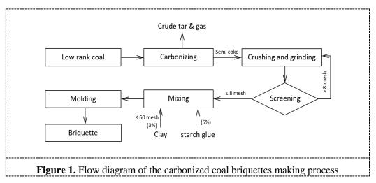
The composition of the briquette mixture consisted of charcoal 92%, filler 3%, and binder 5%. The use of filleris intended to absorb gas emissions and to reduce the fly ash phenomenon during the cooking process. Meanwhile, the use of binder is intended to provide strength to the briquettes so that they are not easily destroyed during transportation, storage, and use[5]. The last step of the briquette making process was the briquettes molding, which was conducted manually.
