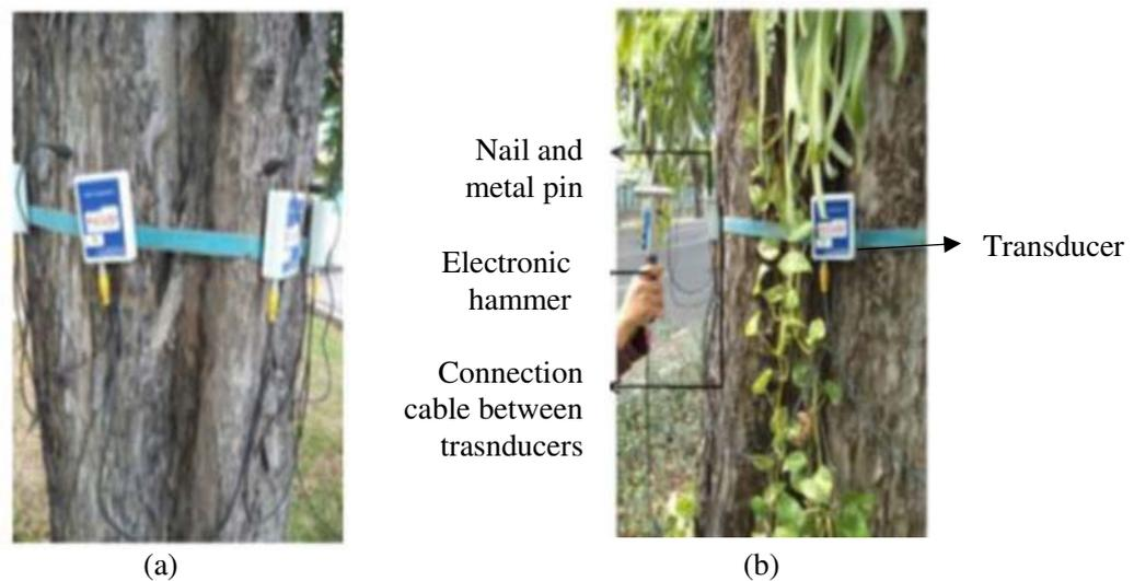
**Figure 2.** (a) Transducers in targeted tree trunk (b) Testing activity by tapping the electronic hammer into the metal pin
