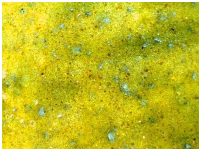
Figure 3. Microstructure of samples based on silicone and phenol-formaldehyde resin powder (2: 1) with the addition of silicon carbide in an amount of 1% mass (x100).
