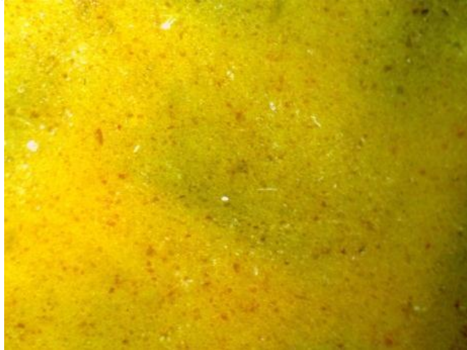
Figure 2. Microstructure of samples based on silicone and phenol-formaldehyde resin powder (2: 1) without silicon carbide additives (x100).
