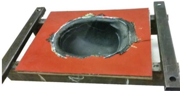
Figure 3. Mould with the poured binder
