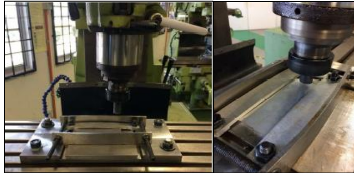
Figure 2. Setup of tool pin profile to performed FSW process [3].
