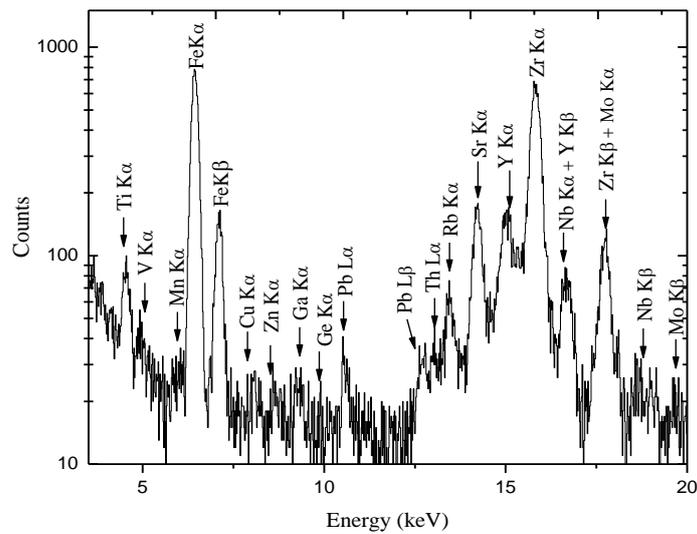
Fig 3. XRF spectrum of fly ash collected from Guru Nanak Dev thermal power plant.
