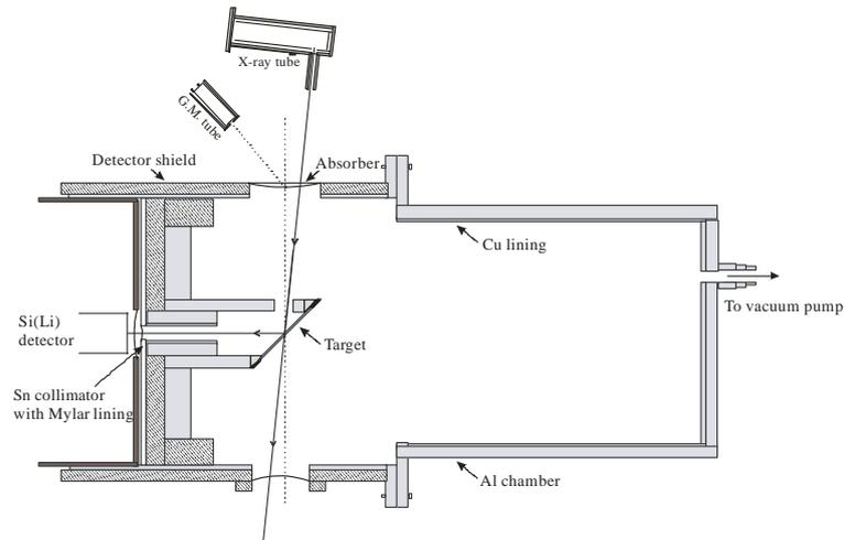
Fig 2. X-ray tube based geometry in the reflection mode.
