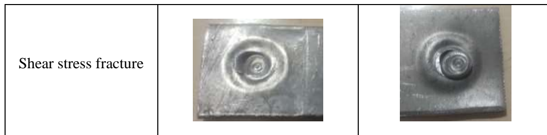
Figure 6. Images of failure surfaces which is described by the failure mode of the test specimens.
