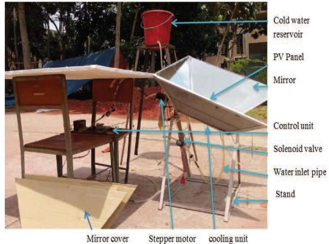
**Figure 2.** The constructed mirror reflected solar panel.
