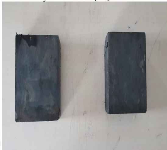
Figure 2. Square magnets of strength 2T.
