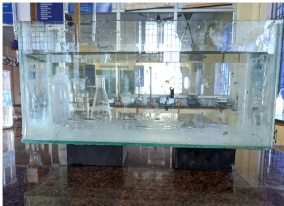
Figure 4. Preparation of Magnetized water for 2T strength.
