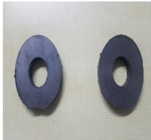
Figure 3. Circular magnets of strength 0.986T.
