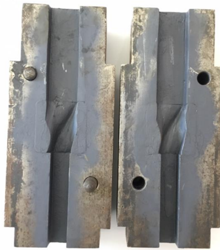
Figure 1. Twist extrusion die.
