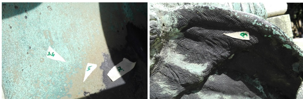
Figure 2. The different type of corrosion products on the surfaces of status. Right image shows a black and porous green layer, left image shows the continuous green and yellow-brown layer with a black covered area.
