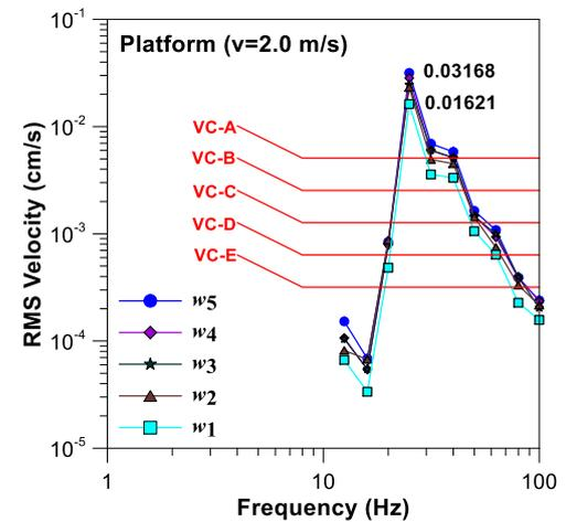
Figure 6. RMS platform vibration spectra.
