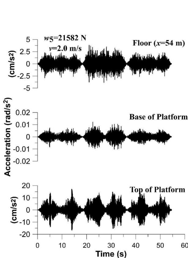
Figure 4. Simulated dynamic time history responses of floor system and platform.
