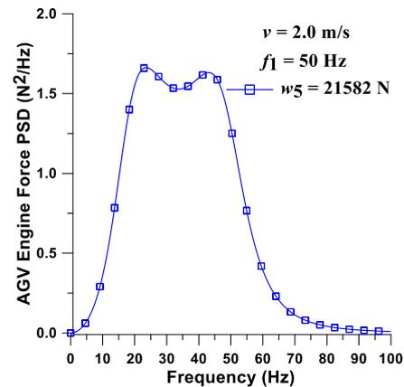
Figure 2. Dynamic engine force spectrum.
