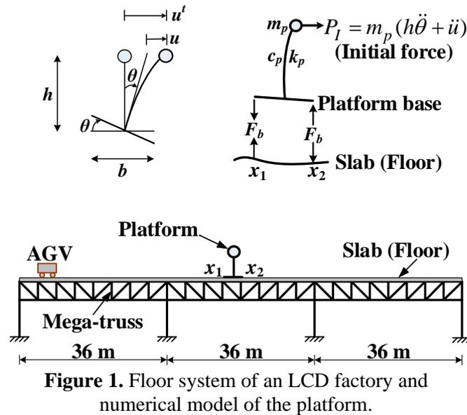
Figure 1. Floor system of an LCD factory and numerical model of the platform.
