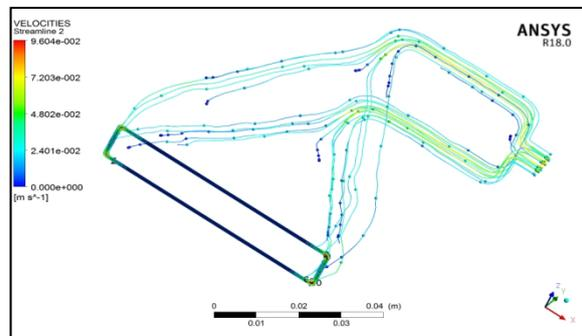
**Figure 8.** Cloud map of velocity distribution in shell flow channel.
