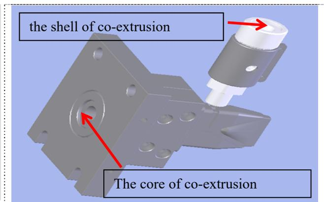
**Figure 2.** The 3D design schematic of co-extrusion die head.
