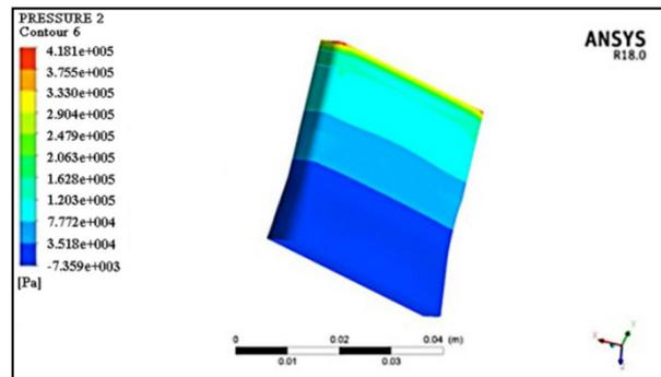
**Figure 18.** Pressure change cloud chart of core material.
