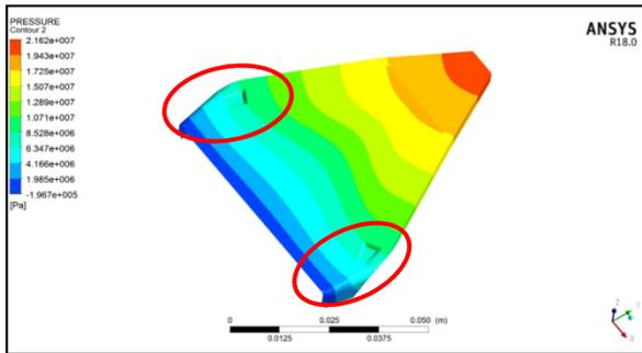
**Figure 11** The pressure field at the exit of damper in a small range at the upper part of bending zone.
