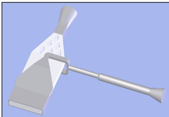
**Figure 3.** CREO modeling diagram of inner and outer layer flow channel.
