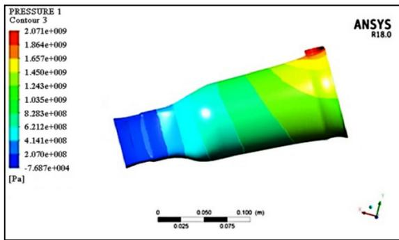
**Figure 17.** Pressure change cloud chart of shell material.
