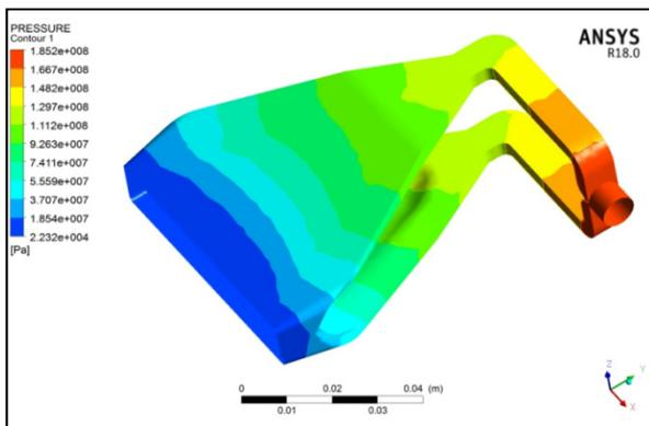
**Figure 9.** Pressure field of shell material.
