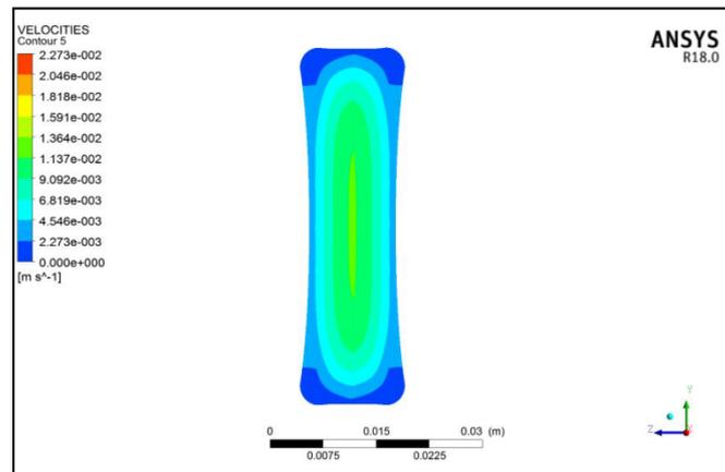
**Figure 21.** Velocity field of die outlet.
