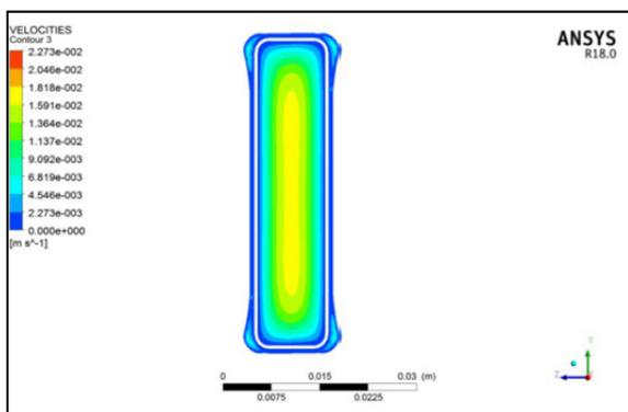
**Figure 19.** Velocity field at the entrance of the die head.
