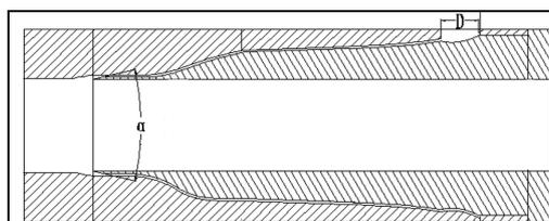
**Figure 16.** Schematic diagram of the overall structure of the die head.
