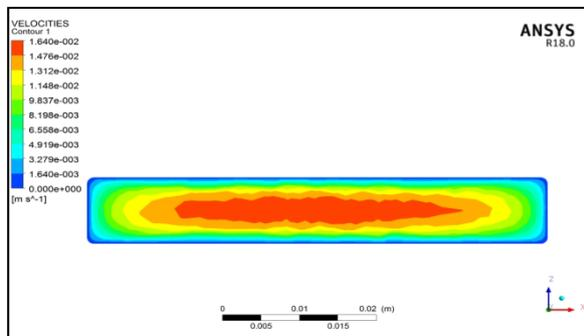
**Figure 7.** Velocity distribution map of core outlet section.
