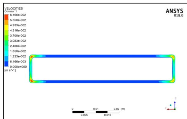
**Figure 10.** Velocity change cloud chart at the outlet of shell flow channel.
