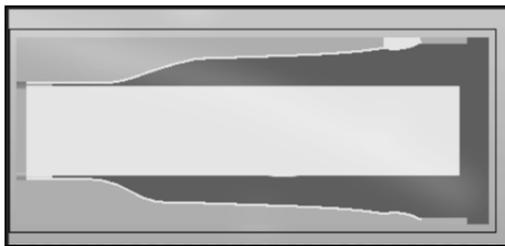
**Figure 14.** Design section diagram of channel of coated co-extrusion die.
