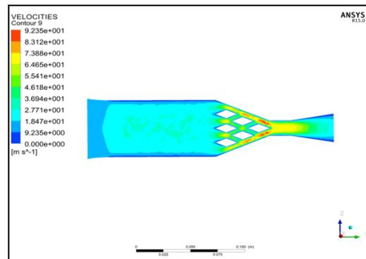
**Figure 6.** Velocity distribution in cross section of core layer flow channel.
