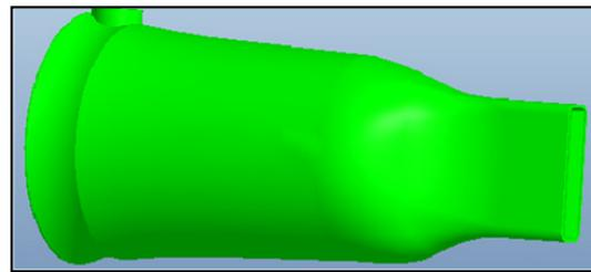
**Figure 15.** The 3D diagram of channel of coated co-extrusion die.
