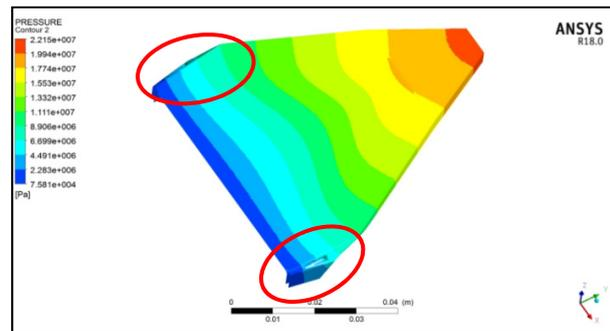
**Figure 12.** The pressure field at the exit of damper with sudden change of four corners.
