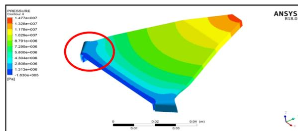
**Figure 13.** Exit pressure field with increasing inclination of bending position.
