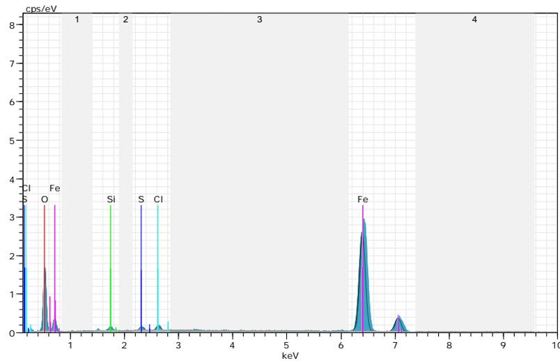
**Figure 4.** Energy spectrum analysis chart for corrosion products.
