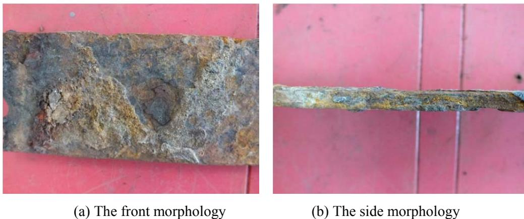
**Figure 1.** The macro morphology of the corroded flat steel of grounding grid.
