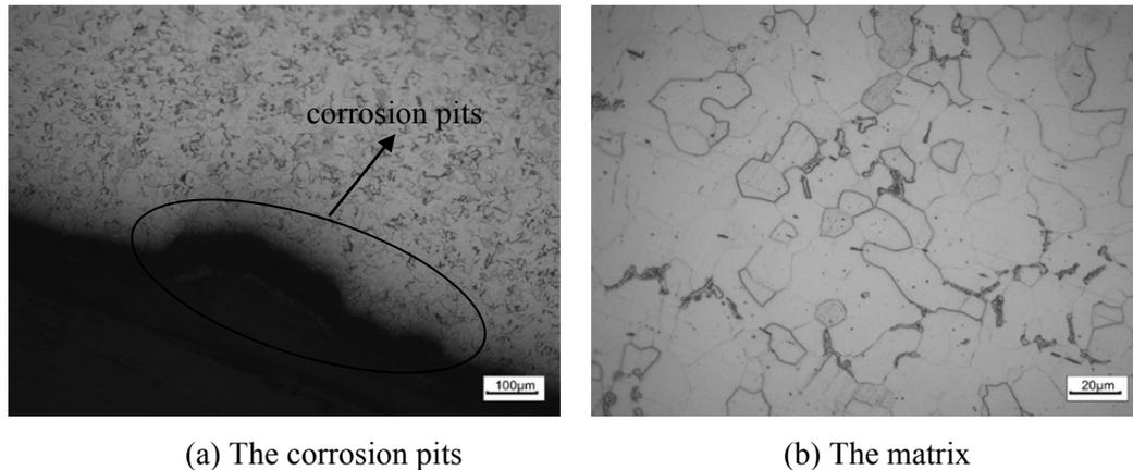
**Figure 2.** The metallographic structure of the corroded flat steel of grounding grid.
