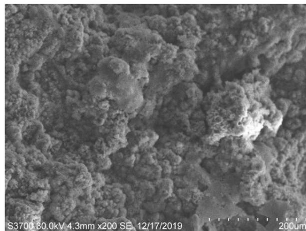
**Figure 3.** The SEM morphology of corrosion products.
