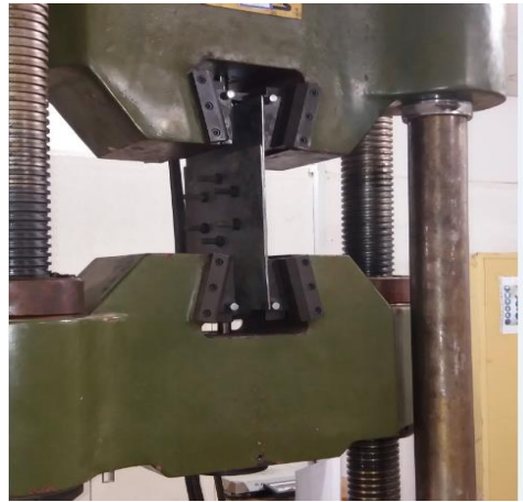
Figure 5. Specimen under tension by computer controlled versatile electronic testing machine.
