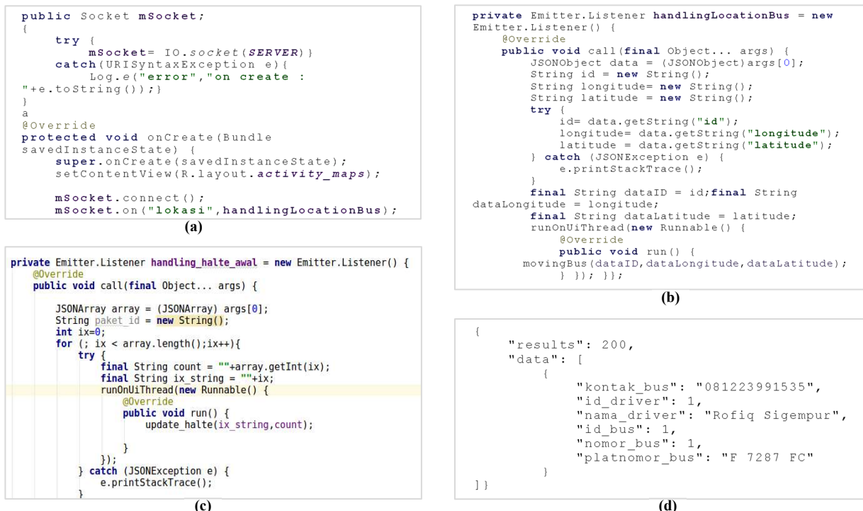
Figure 5 (a) Client socket initialization to enable real time location data exchange; (b) passenger receive screen visualization of driver's location through the JavaScript Object Notation (JSON); (c) segment code to display the number of passengers at the bus stop; and (d) REST API output results in JSON format.
