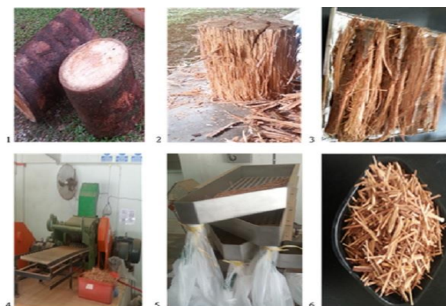
Figure 1. Preparation steps of sago palm bark
