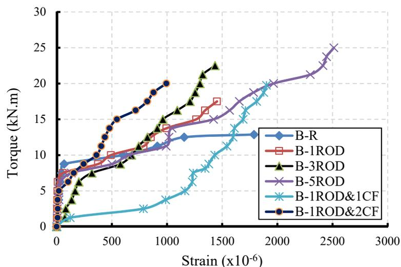
**Figure 10.** Torque-strain in longitudinal bars.
