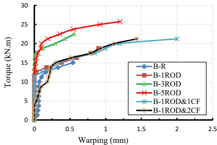
**Figure 9.** Torque-warping behavior for tested beam specimens.
