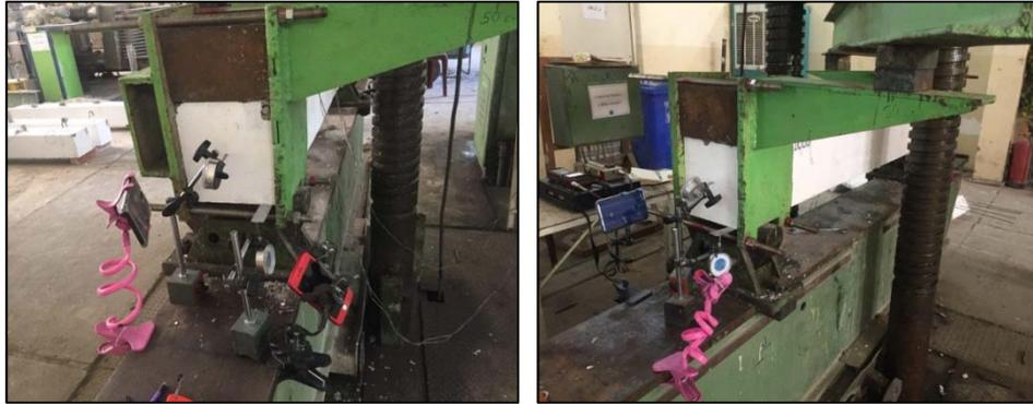
**Figure 5.** Locations of dial gauge and test setup of all considered beam specimens.
