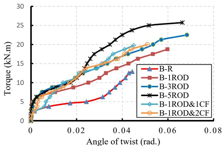
**Figure 8.** Torque-angle of twist response for tested beam specimens.
