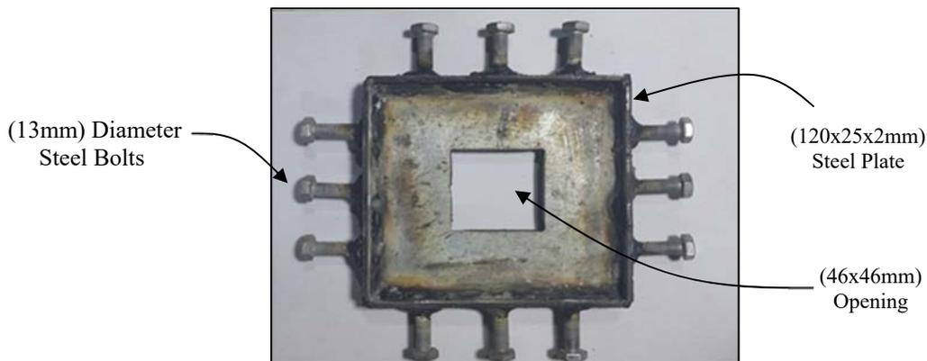
**Figure 4.** Steel diaphragm with rectangular opening.
