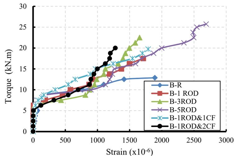
**Figure 11.** Torque-strain relationship for stirrups.
