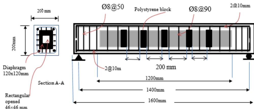
**Figure 3.** Reinforcement and details of tested beam (B-5ROD).
