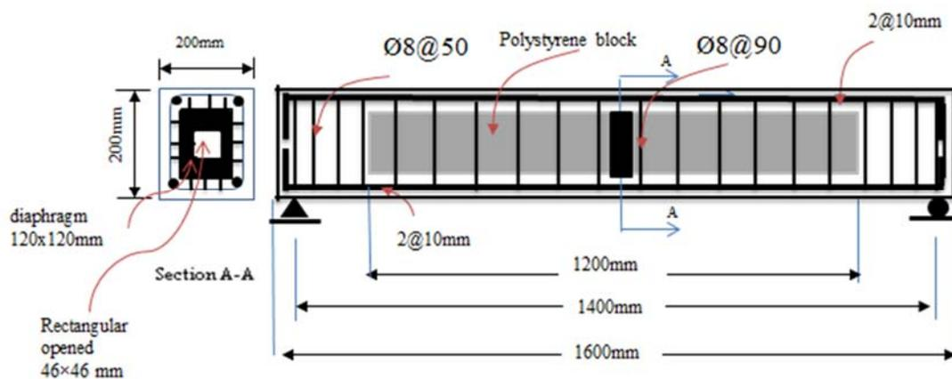
**Figure 2.** Reinforcement and details of tested beam (B-1ROD).
