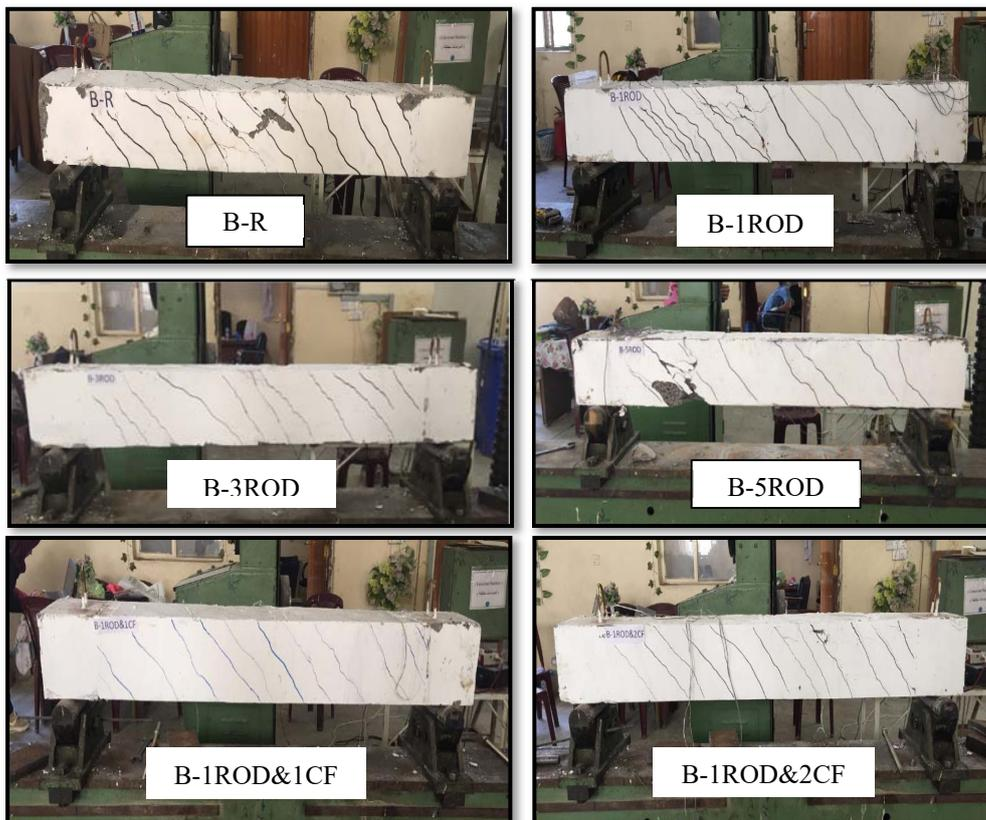
**Figure 7.** Torsion mode of failure for tested beams.
