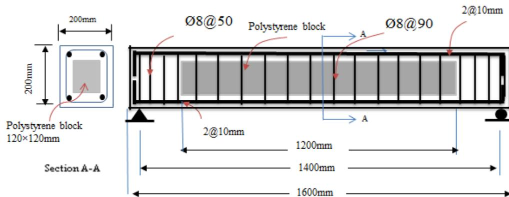
**Figure 1.** Reinforcement and details of tested Beam (B-R).
