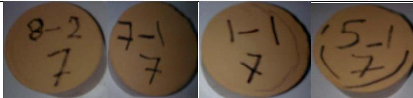
**Figure 11.** Samples burned to 750 ° C
