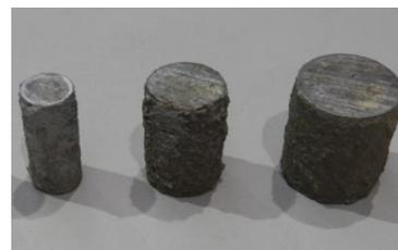
**Figure 4.** Steel inclusions with epoxide layer ( $\phi = 20, 30, 40$  mm).
