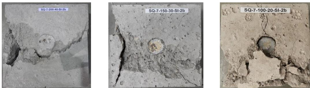
**Figure 10.** Failure of specimens with *SI*-interface (Images size ratio 1:0.75:0.5).
