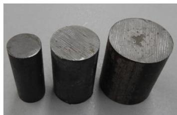
**Figure 3.** Steel inclusions ( $\phi = 20, 30, 40$  mm).
