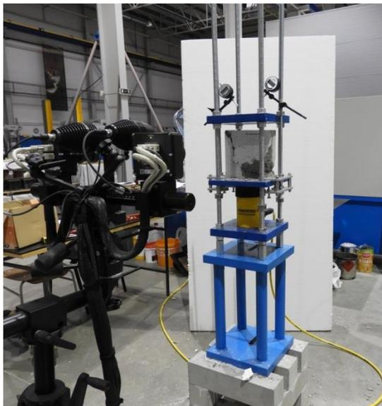
**Figure 5.** Arrangement of the uniaxial compression test.
