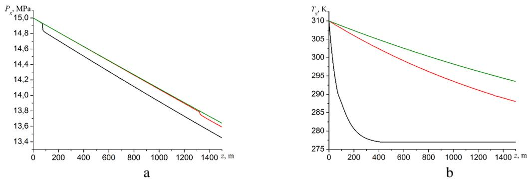
**Figure 2.** Change of pressure (a) and temperature (b) of the gas along the outlet pipe at different thicknesses of insulation:  $\delta_{pp}=0.5$  cm – red line;  $\delta_{pp}=1$  cm – green line; without insulation – black line
