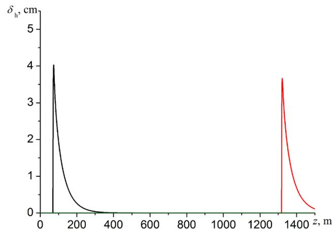
**Figure 3.** Change in the thickness of gas hydrate along the discharge pipe at different thicknesses of insulation:  $\delta_{pp}=0.5$  cm – red line;  $\delta_{pp}=1$  cm – green line; without insulation – black line.
